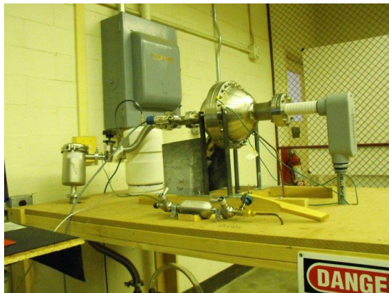
Figure 1.2. A picture of Virginia Tech's Fusor (left) and the field lines associated with the ion acceleration in two dimensions (right).
