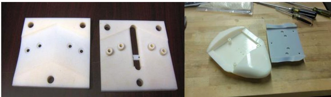
Figure 3.3: Inner and outer clamshell fuselage pieces (outer on right; inner on left)
