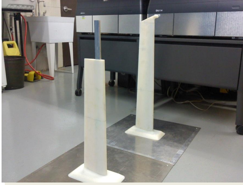
Figure 3.6: Strut on which test article was mounted. (front of picture)
