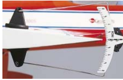
Figure 40 - Control surface deflection meter
