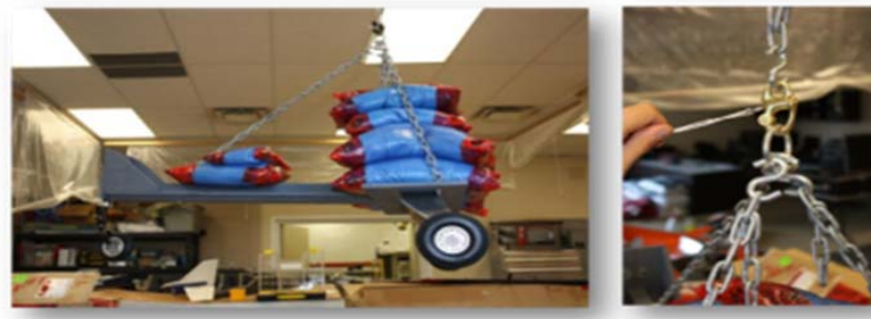
Figure 22- Landing Gear Drop Test Rig 12
