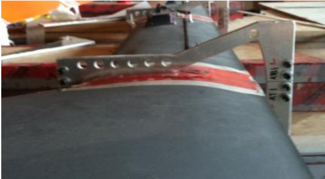
Figure 3.3: Aft wing outer rib attachment
