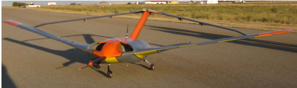
Figure 17- Tricycle Landing Gear on GSRPV
