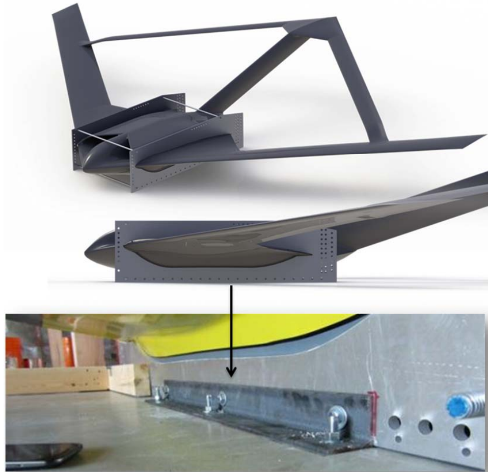
Figure 34- Fuselage concept (top); Steel angled bracket for ground restraint (bottom)
