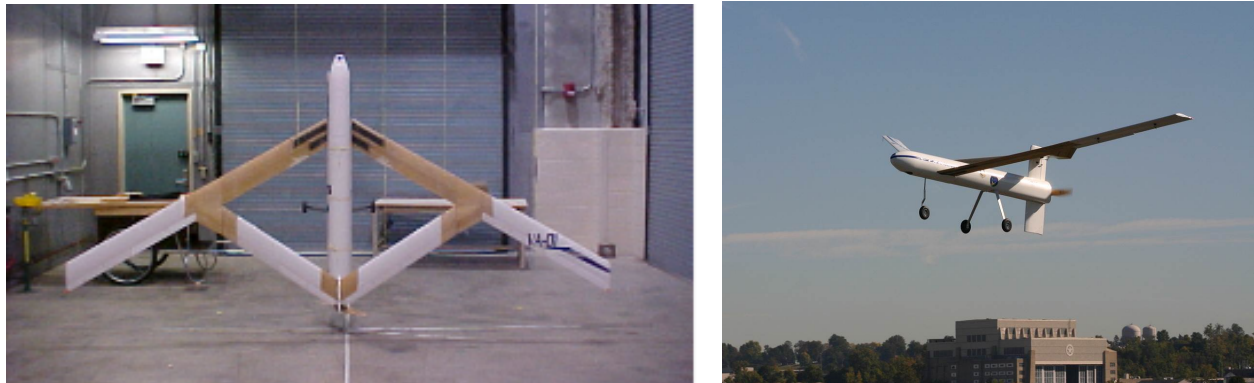
Figure 1.6: VA-1 top profile view (left); VA-1 remote-controlled joined-wing aircraft (right). McClelland, W.A., Inertia Measurement and Dynamic Stability Analysis of a Radio Controlled Joined-Wing Aircraft , Master's thesis, Graduate School of Engineering and Management, Air Force Institute of Technology, 2006. (Source approved for public release by U.S. Government )
