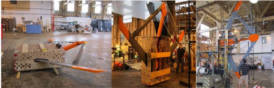
Figure 38- Bifilar pendulum test configuration (GSRPV) for yaw (left), roll (middle), and pitch (right) 10,12
