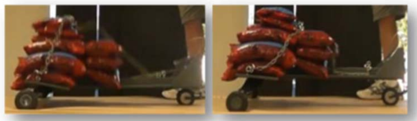
Figure 23-Landing Gear at Impact (Left); Landing Gear after Test (Right) 12
