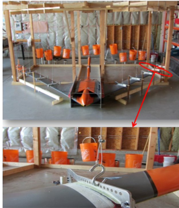
Figure 3.5: Pulley system (top); Zoomed in view of attachment to outer ribs (bottom)
