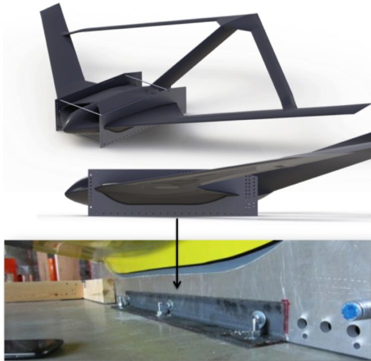
Figure 3.4: Fuselage cage with steel bracket
