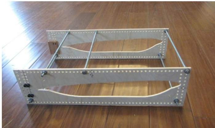
Figure 25- Fuselage cage used to prevent rotation of the RPV during load tests
