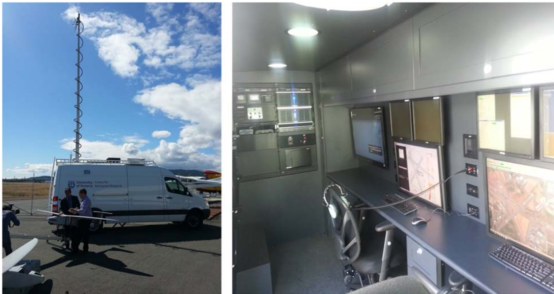
Figure 44 – Mobile Ground Station (Left), Internal (Right)
