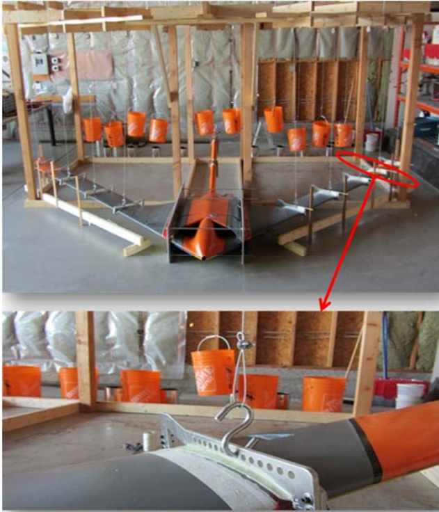
Figure 36 –Full static loading set up (top); Zoomed in view of load application
