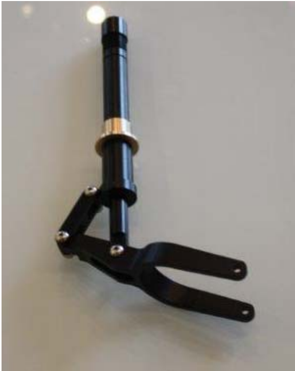
Figure 16- Custom Designed Oleo Strut for Nose Gear
