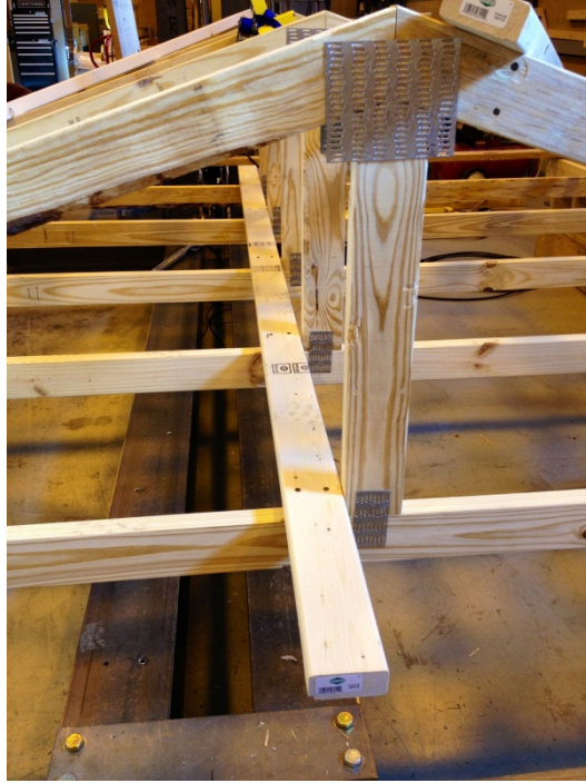
Figure 2-6: Bottom chord bracing configuration
