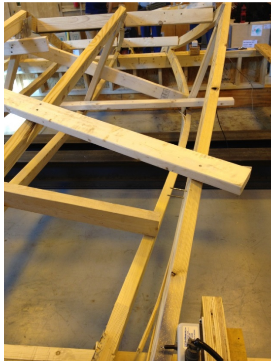
Figure 3-44: Failure in the bottom chord of the truss
