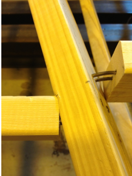
Figure 3-4: “Pinching” action of the in-between bracing
