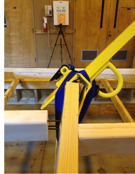
Figure 3-3: Failure in the PFA (back)
