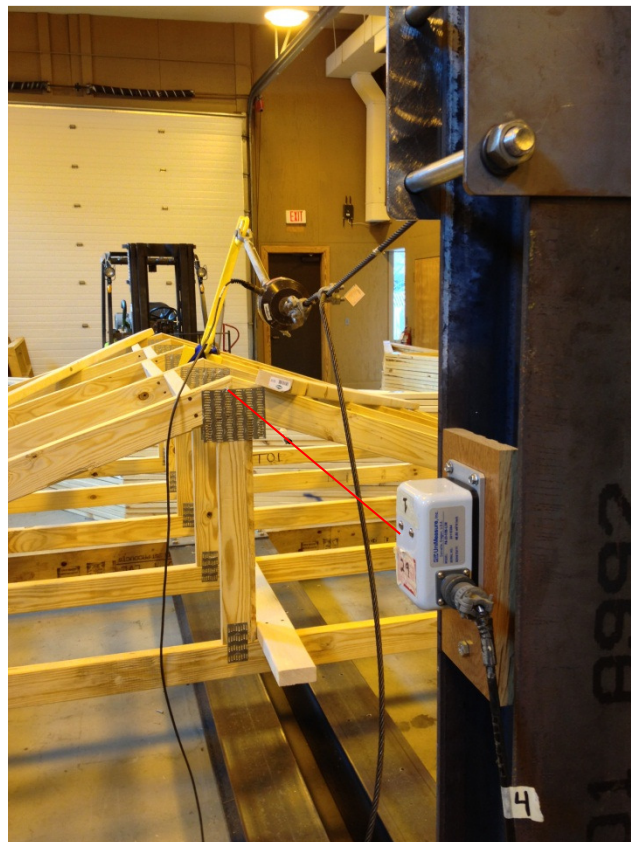
Figure 2-15: String potentiometer attached to the peak of the truss
