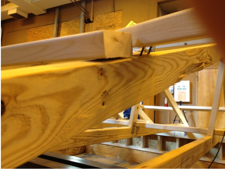
Figure 3-6: Withdrawal of the bracing with PFA
