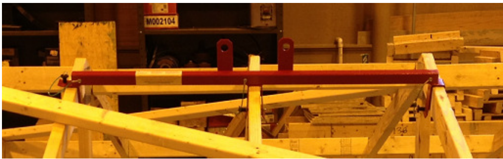
Figure 2-9: Spreader bar anchor
