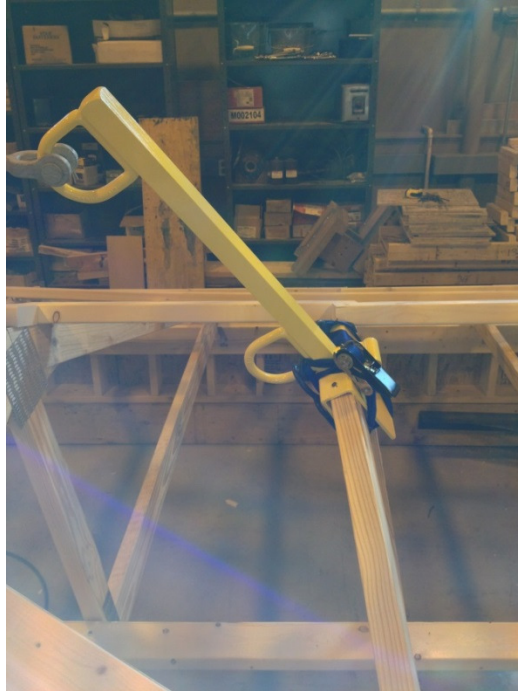
Figure 3-8: PFA after testing with on top bracing
