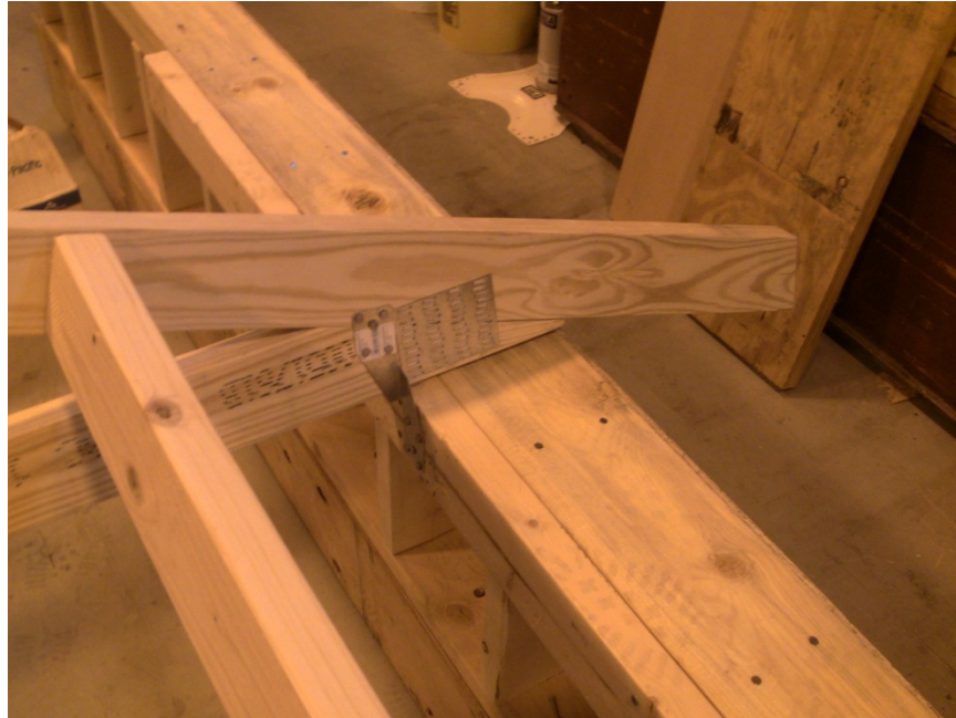
Figure 2-11: Hurricane strap application for testing
