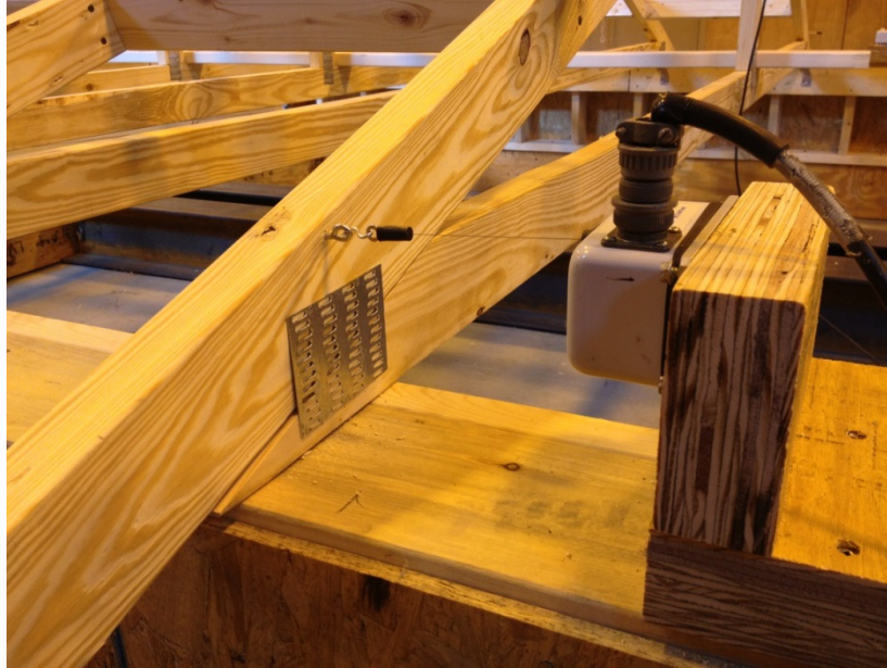
Figure 2-14: String potentiometer at truss-wall connection
