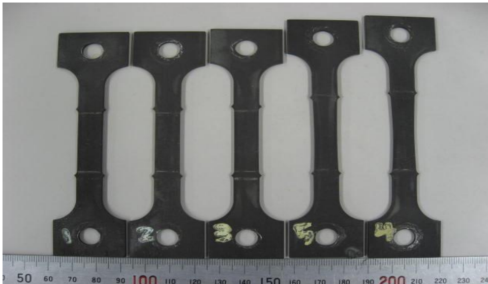
Figure 3.1. Dog bone type specimens after tensile test
