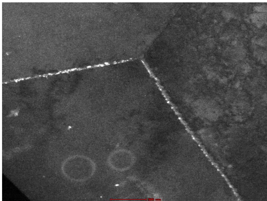
Figure 4.3. STEM dark-field micrograph of Fe 2 Nb Laves phase precipitates found on a triple junction
