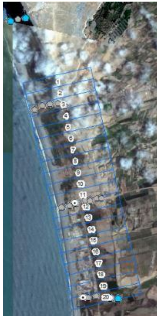
Figure 3.3. Overview of the affected area at Canchamana showing bin numbers, SPT and MASW test locations (Background image from Google Earth)
