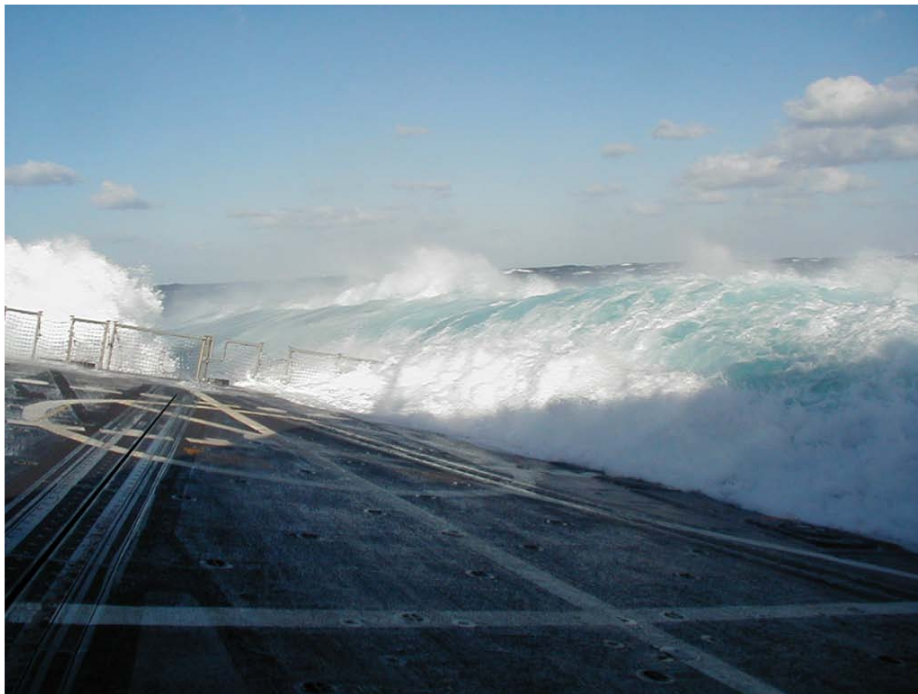
Figure 1-6. A large roll angle, coupled with waves, results in deck submergence and wetness on the flight deck, aft on a U.S. naval vessel
