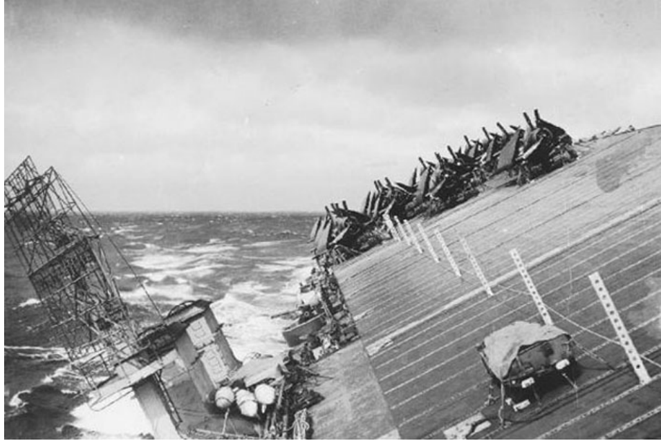
Figure 1-5. Large roll angle experienced by the USS Cowpens , during Typhoon COBRA (Halsey's Typhoon), 18 December 1944 5 . The ship experienced up to 47 degrees of roll.
