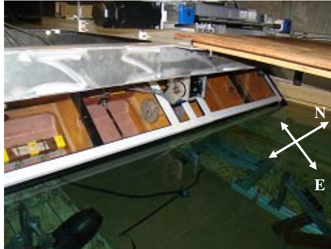
Figure 4-8. Model rolled, while attached to the 3DoF mechanism with submerged PIV laser probes (bottom right, facing West) and camera (bottom left, facing North) shown
