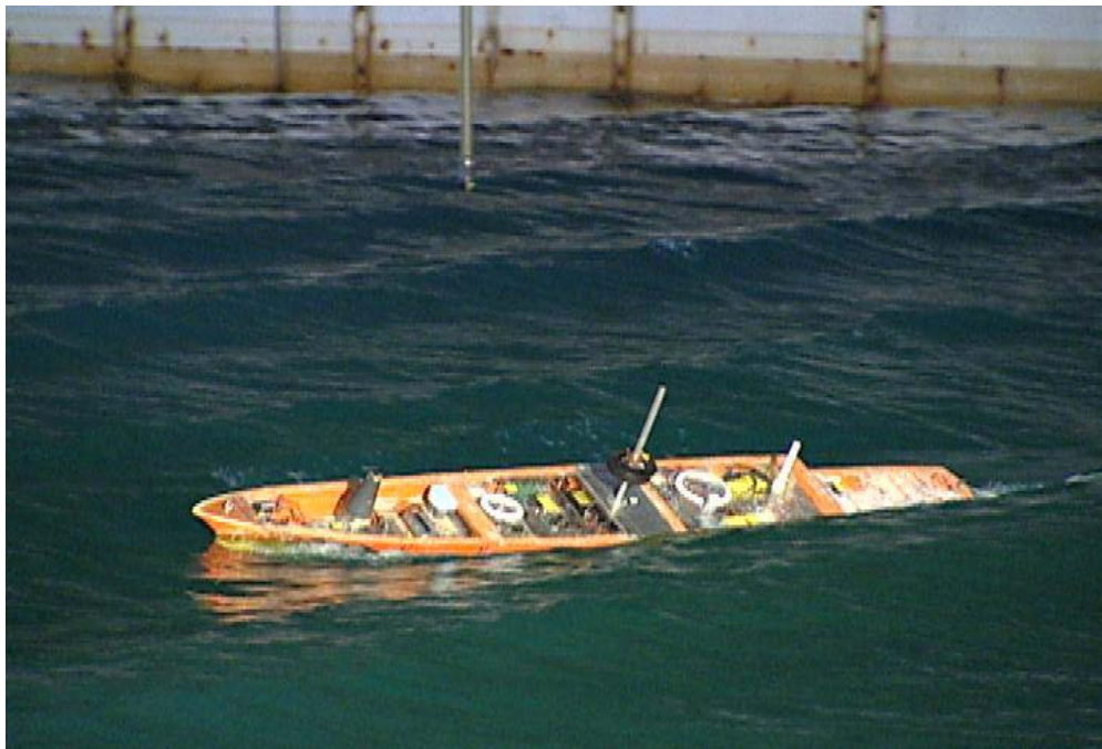
Figure 1-2. A traditional notional naval combatant model (DTMB Model #5514) in hurricane sea conditions, experiencing a large roll angle with bilge keel emergence on the starboard side and deck submergence on the port side 2
