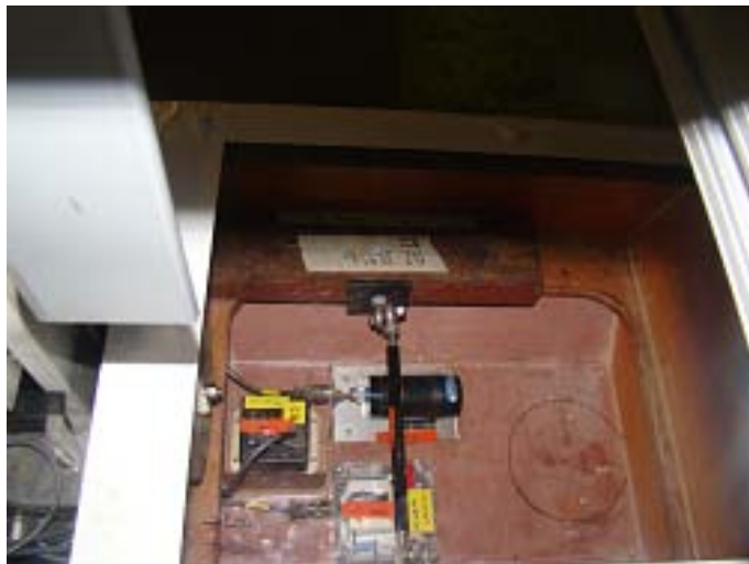
Figure C-10. Displacement gyroscope (clear box) and rate gyroscope (black cylinder) in the model, with topside configuration and plexiglass deckplating installed
