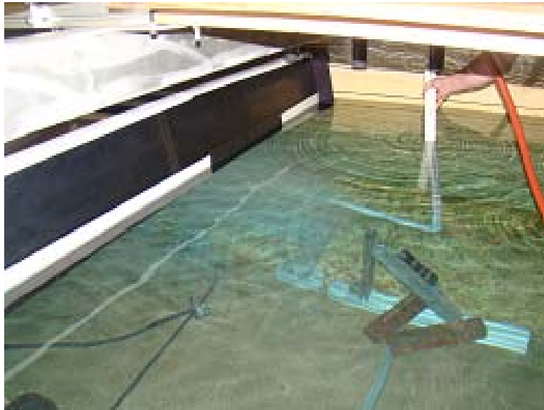
Figure 4-11. Custom designed seeding mechanism shown being used to seed particles in the PIV measurement plane near the hull
