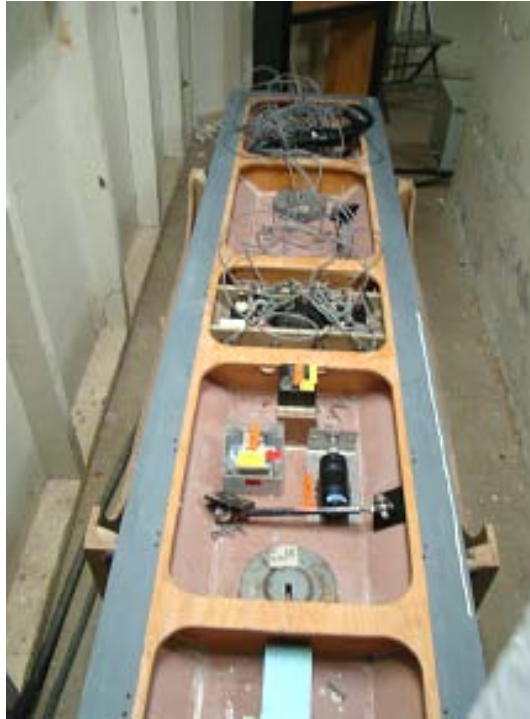
Figure C-9. DTMB Model #5699 with topside removed, viewed from forward looking aft, displacement and rate gyroscopes used to obtain motion measurements are shown in foreground (in the near-field compartment)
