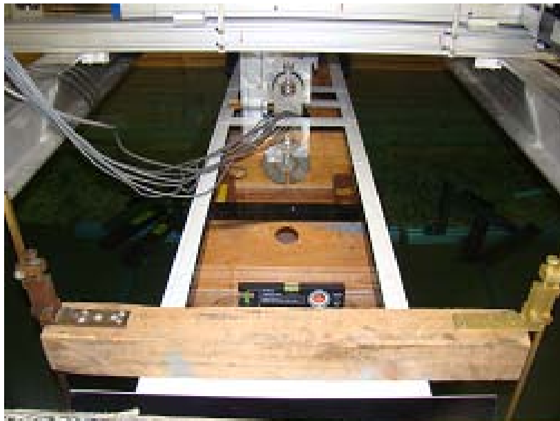
Figure 4-13. Hook-gages and inclinometer used to check the heel angle of the model
