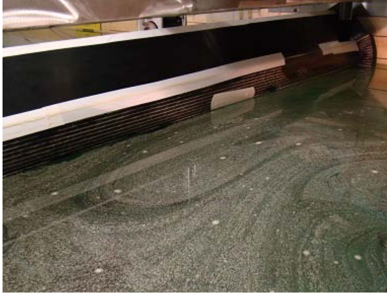
Figure 4-10. Model shown in roll motion (without bilge keels), with PIV particles on the free surface after seeding
