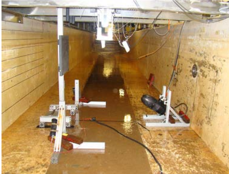
Figure 4-9. PIV set-up in the NSWCCD 140 ft basin, looking East, with camera (right) and calibration target with laser probes (left) shown
