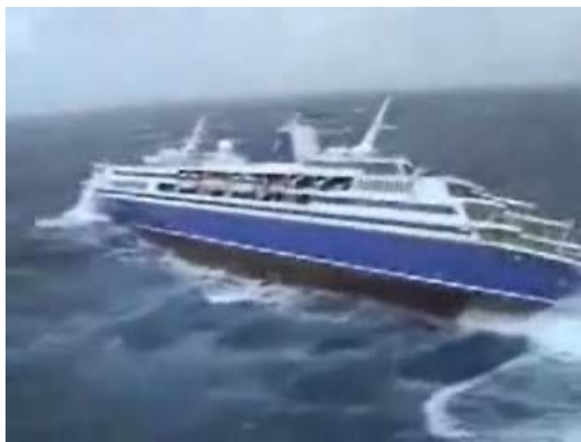
Figure 1-4. Cruise ship Voyager in a storm in the Mediterranean, as viewed from a helicopter, experiencing large roll motions, resulting in bilge keel emergence 4
