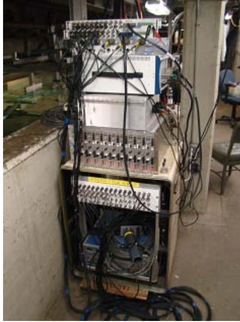
Figure 4-12. Data collection interfaces, not including PIV, ultrasonic wave probes (top), gyroscopes (top middle), bilge keels (lower middle), and Kistler dynamometer (lower)
