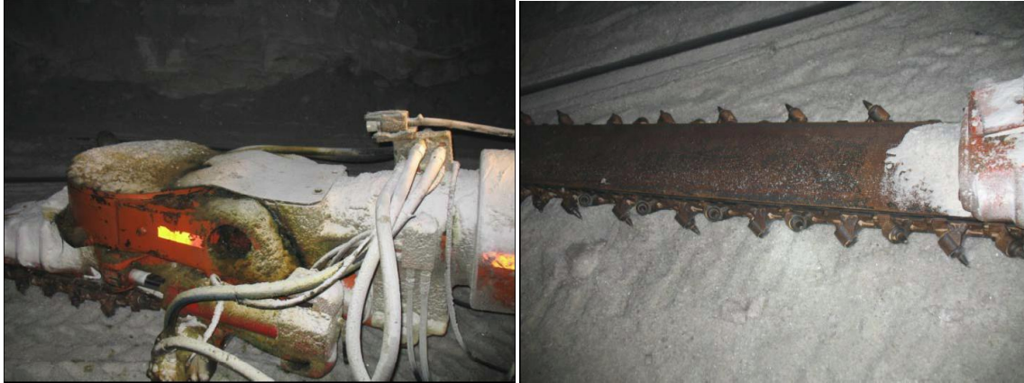
Figure 3.2: Joy Undercutter (Right, Top View) with Methane Sensor (Left, Side View)
