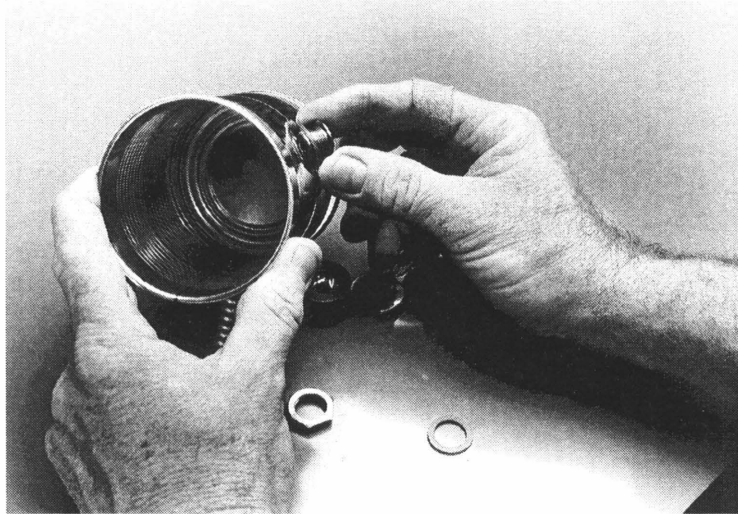
Figure 24. Inserting the thermocouple receptacle and gasket.
