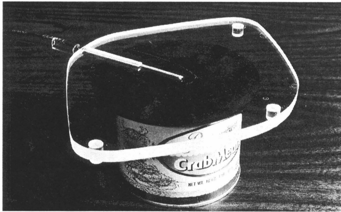
Figure 33. A can leak detector which uses vacuum to draw air out of the suspect can. Leaks are identified by bubbles viewed through the transparent plate as they rise through water previously poured into the can.
