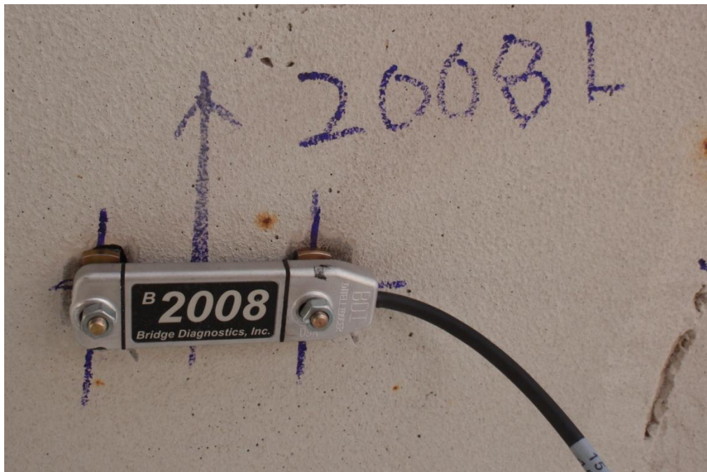
Figure 19 – Strain Transducer 2008 on outside of Seabreeze Bridge
