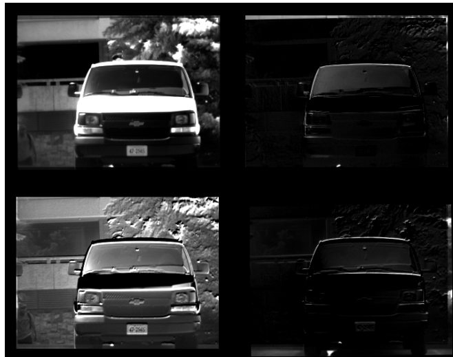
Figure 80: The stokes parameters calculated from the images in Figure 79. (top left) S_0 . (top right) S_1 . (bottom left) S_2 . (bottom right) S_3 .
