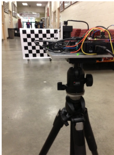
Figure 47: An image showing the test setup used to determine pixel shift at various distances.
