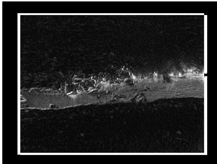
Figure 76: The degree of polarization of Stroubles Creek viewed perpendicular to the sun.
