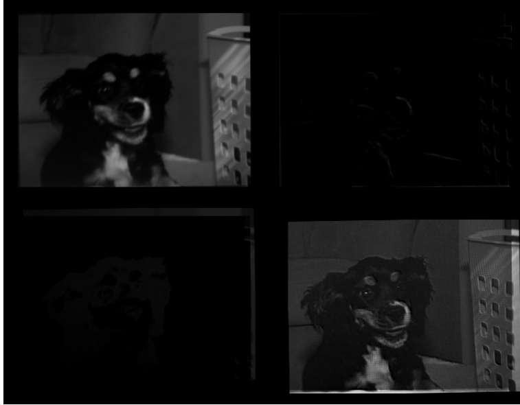
Figure 58: Stokes images of a -45^\circ polarized LCD monitor. The images are shown on a scale of 0 to 1, truncating any negative values for visualization purposes. (top left) S_0 , (top right) S_1 , (bottom left) S_2 , (bottom right) S_3 .
