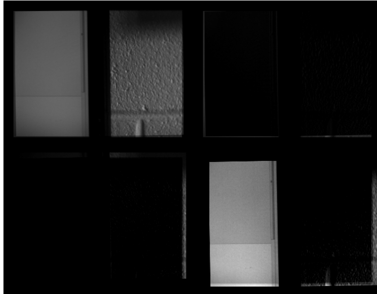
Figure 60: Stokes images of a -45^\circ polarized LCD monitor and cinderblock wall. (top left) S0, (top right) S1, (bottom left) S2, (bottom right) S3.
