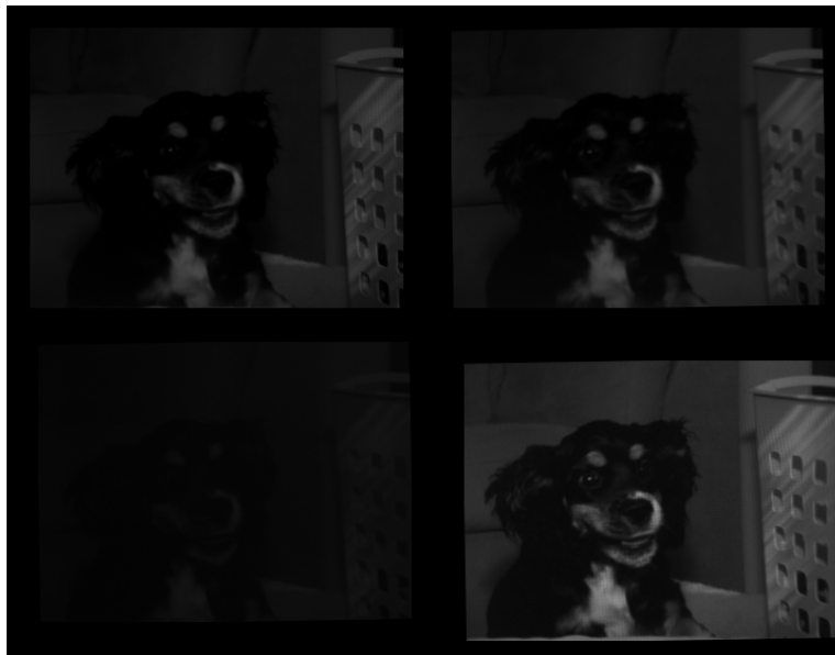
Figure 57: A set of raw images of a -45^\circ polarized LCD monitor. (top left) Camera 0, (top right) Camera 1, (bottom left) Camera 2, (bottom right) Camera 3.
