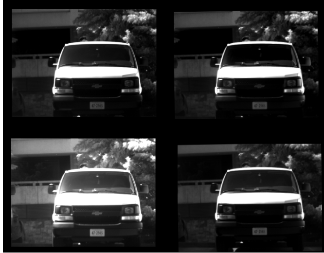
Figure 79: A set of polarized images of a typical van. (top left) Horizontally polarized. (top right) Vertically polarized. (bottom left) 45^\circ polarization. (bottom right) -45^\circ polarization.
