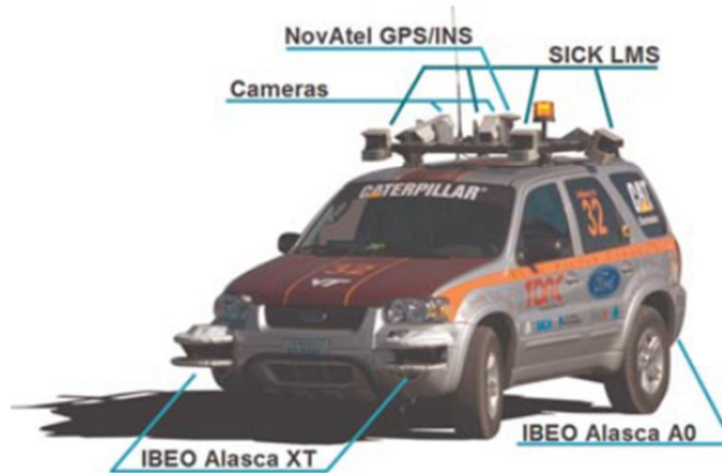
Figure 2: The Victor Tango Ford Escape hybrid, Odin, with sensors labeled [5].
