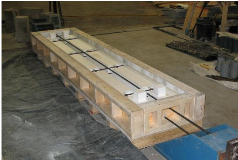
Figure 3-53: Foam was placed directly into the form for DS-2.
