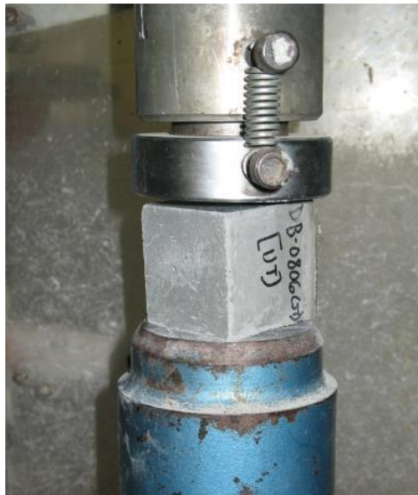
Figure 3-3: Testing compressive strength of UHPC using 2 in. cubes.
