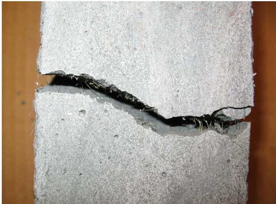
Figure 6-25: Failure crack of SP-C1 (top of web).
