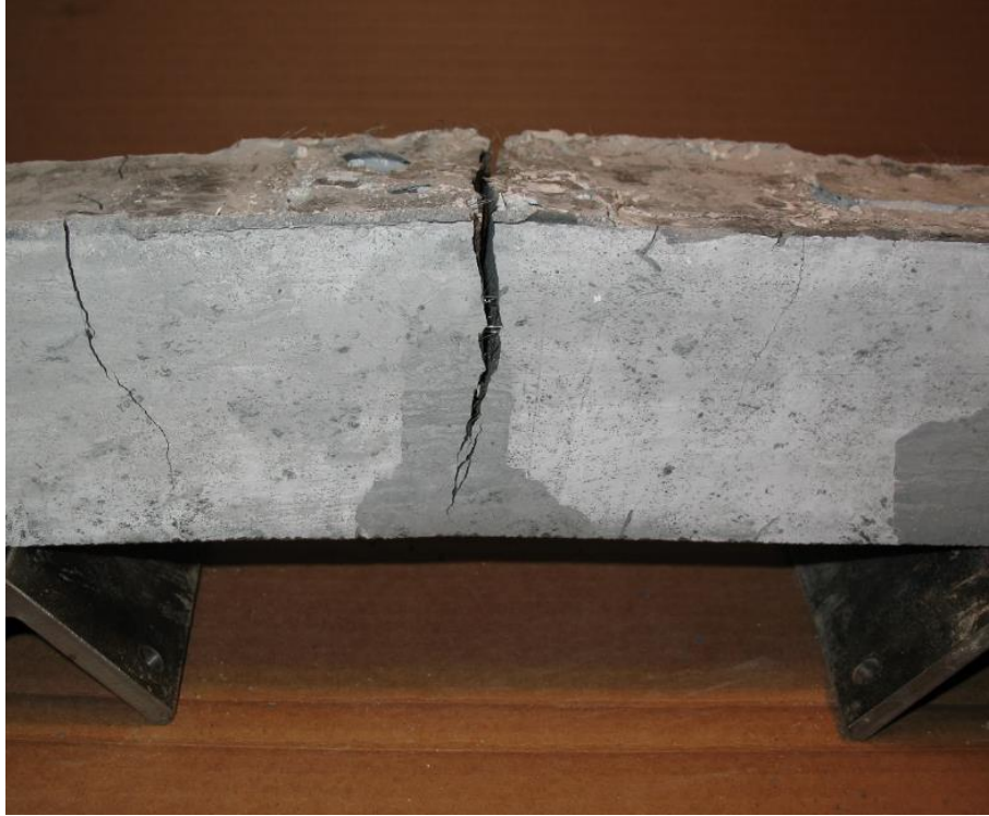
Figure 6-24: Failure pattern of UD-B2 (bottom of web).
