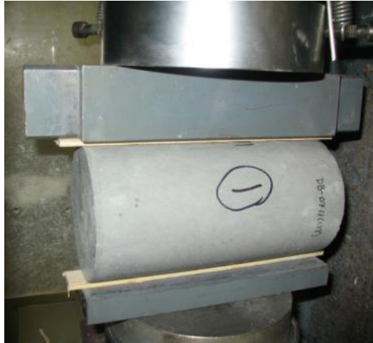
Figure 3-5: Split cylinder test set-up.
