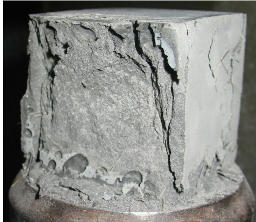
Figure 7-3: A lack of fibers in cubes resulted in sudden compressive failures.
