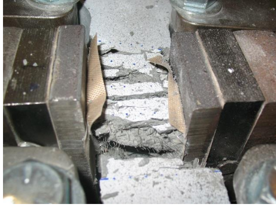
Figure 5-23: Teflon-coated tape was damaged during testing (UT-I, 0.4f t -1).
