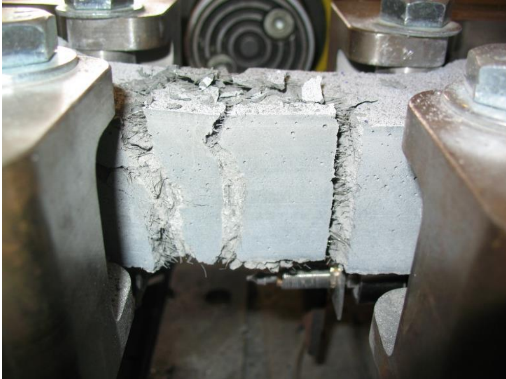
Figure 5-20: Vertical cracking was common with UT-I failures (0.4ft-2).
