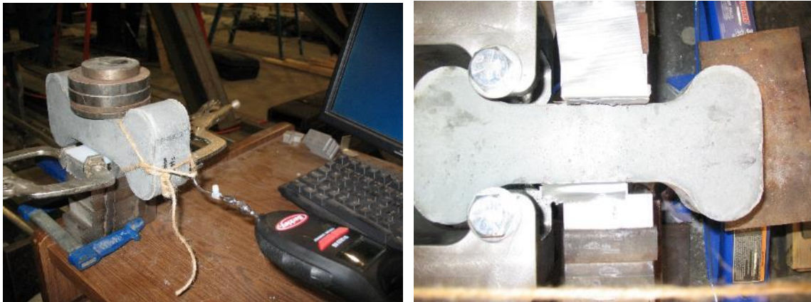
Figure 3-27: Coefficient of static friction was determine experimentally.
