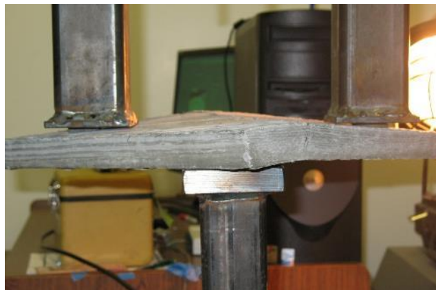
Figure 4-6: Cracks first formed in the side with dominant tensile stresses.
