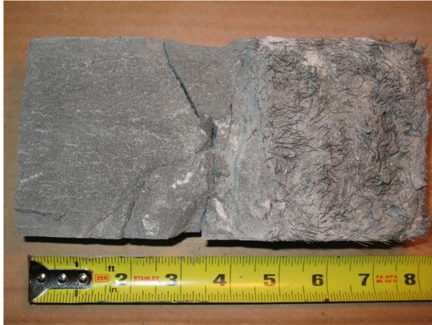
Figure 7-6: Fibers were observed to be concentrated in the bottom 3 in. of an 8 in. high cylinder as the most extreme case of fiber settling (DS-2B).
