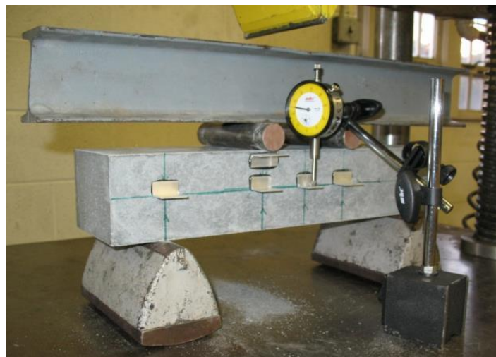
Figure 3-7: Preliminary flexure prisms test set-up.
