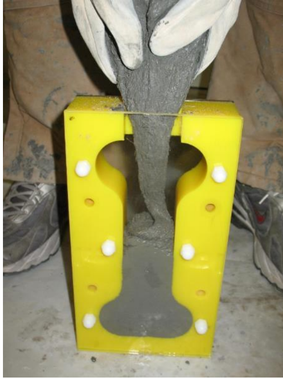
Figure 3-24: UHPC was added vertically into the direct biaxial dog bone test forms.
