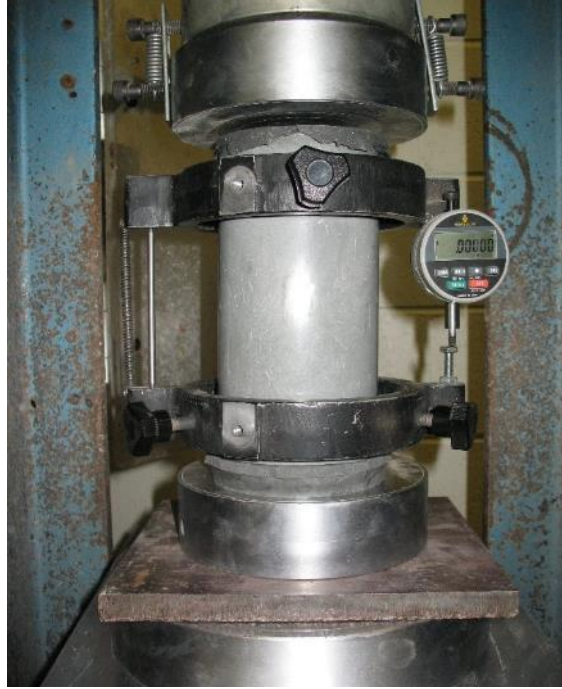
Figure 3-4: The compessometer was used to determine the elastic modulus.
