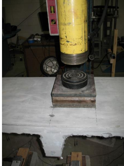
Figure 3-70: An 8 in. square bearing pad and steel plates provided pressure.
