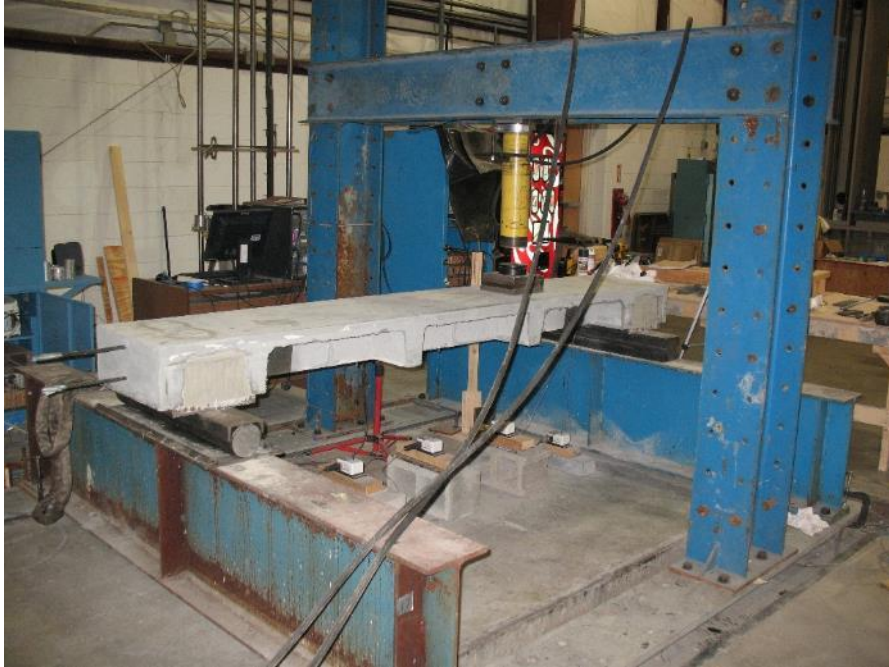
Figure 3-67: A steel frame was constructed to test the deck sections.
