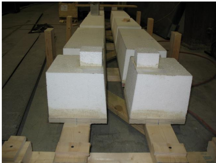
Figure 3-50: Foam was connected to a wooden frame for the upside down placement of DS-1.
