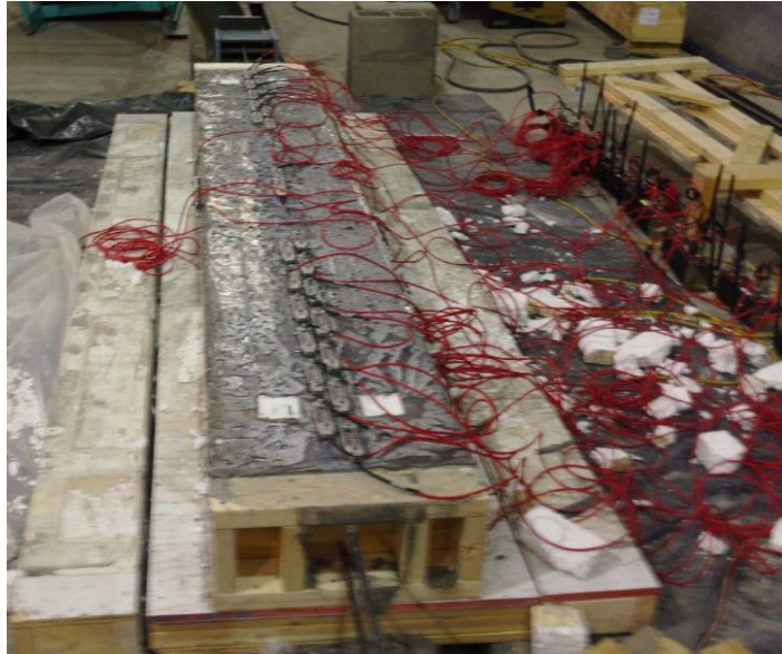
Figure 3-60: BDI gages were attached to DS-2 and measured using the BDI Wireless Structural Testing System as data acquisition.
