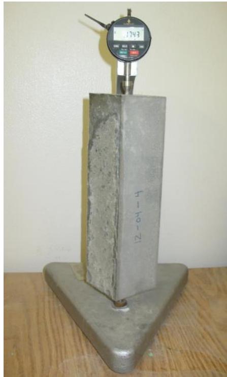
Figure 3-8: Shrinkage was determined by comparing length changes over time.
