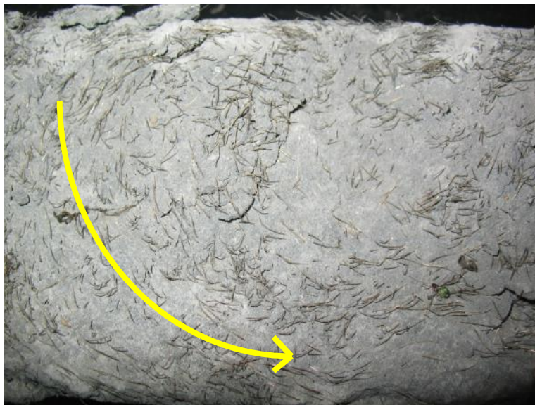
Figure 4-1: Circular fiber orientation in cylinder specimen.
