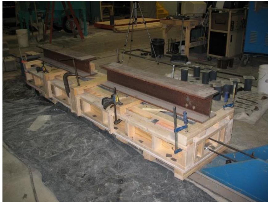
Figure 3-52: The frame was clamped and two steel beams provided additional force along the center section to prevent uplift.
