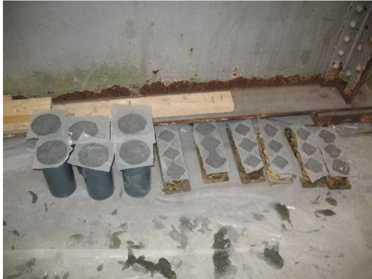
Figure 3-44: Cubes and cylinders were placed to characterize material properties.
