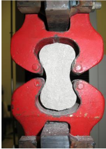
Figure 3-6: Briquet tensile test set-up.
