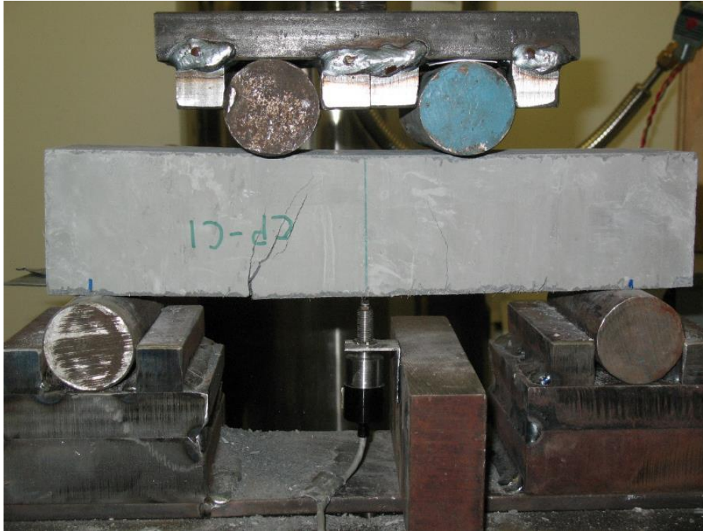
Figure 3-46: Third-point bending test for beams cut from single cells.
