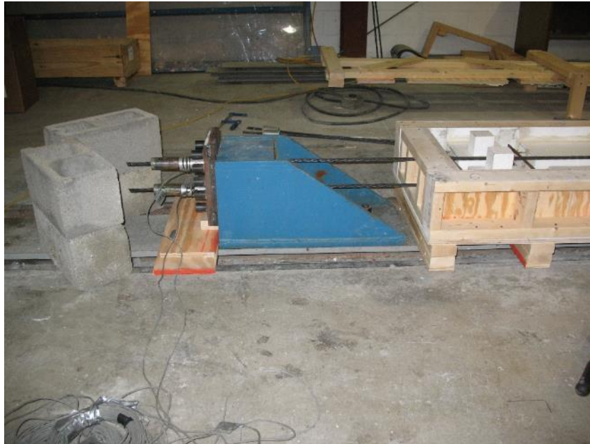
Figure 3-55: A load cell was placed between the steel abutment and a chuck.
