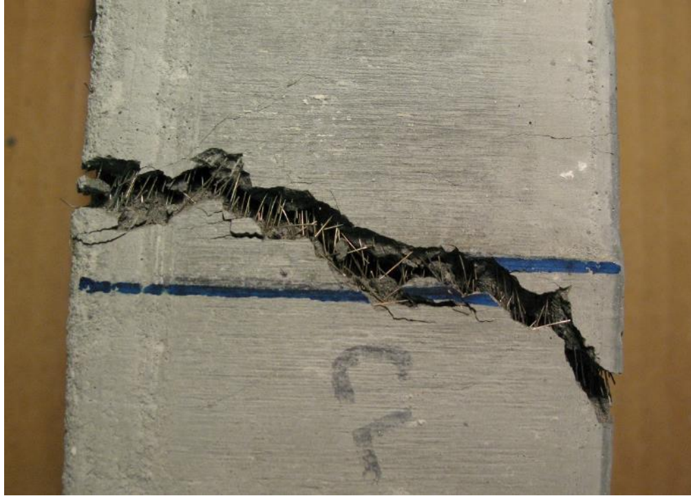
Figure 6-28: Failure crack of CP-D2 (bottom of web).
