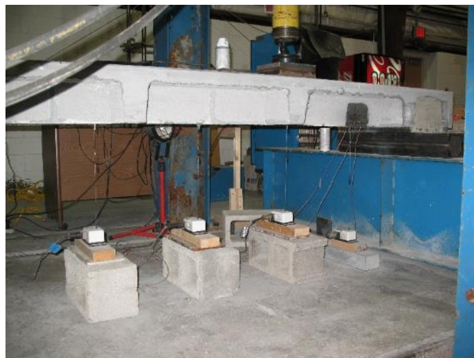
Figure 3-71: Four CETs determined deflection at critical locations.
