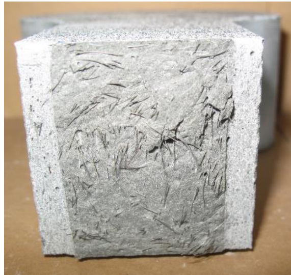
Figure 5-13: Randomized fiber orientation in pure tension (PT) sample for steam treated curing.
