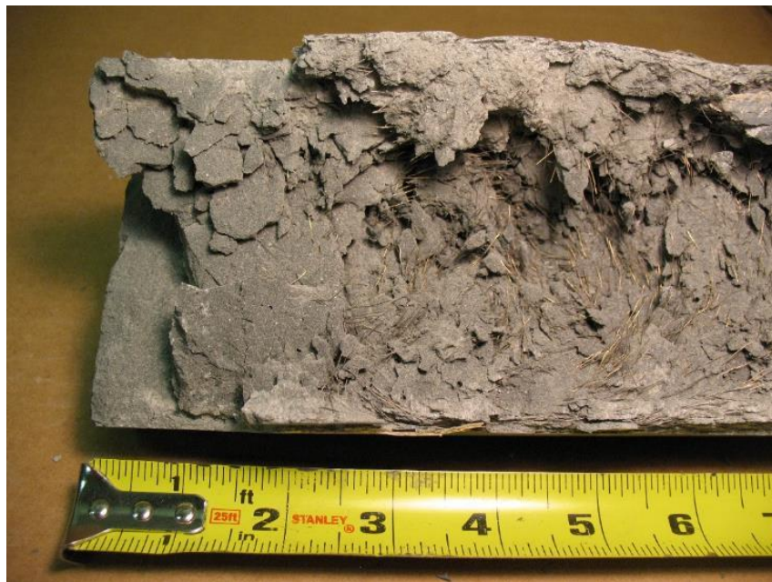
Figure 7-5: Fibers were observed to be sinking approximately 2 in. from the top surface of an 8 in. high cylinder (DS-2A).
