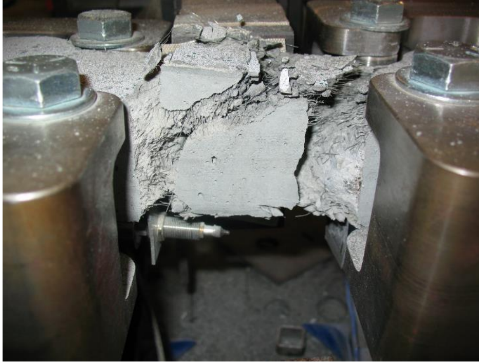
Figure 5-16: Curved failure surface of 0.4ft-3 sample with steam treated curing.
