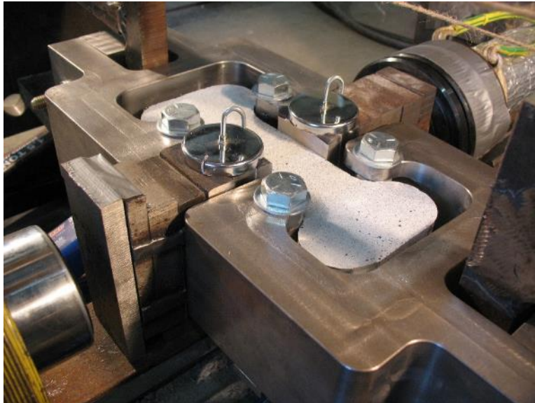
Figure 3-29: Magnets were used to hold free-floating steel blocks in place prior to compression force application.
