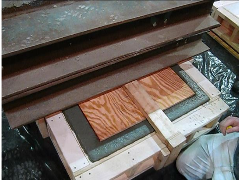
Figure 3-42: Steel beams were placed atop the frame to maintain constant pressure (Photo by K. Halbe).
