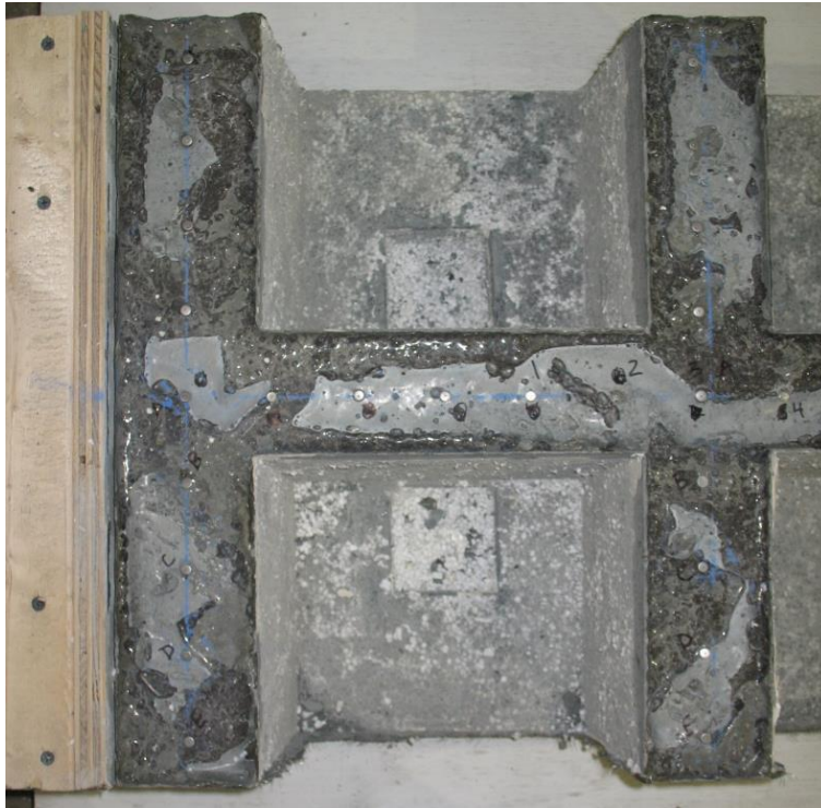
Figure 3-58: DEMEC points were applied to the exposed surface along the centerline of the web.
