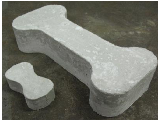
Figure 3-20: Briquet specimen for AASHTO Standard T 132-87 (2004) standard test (lower left) and direct biaxial test specimen (upper right).
