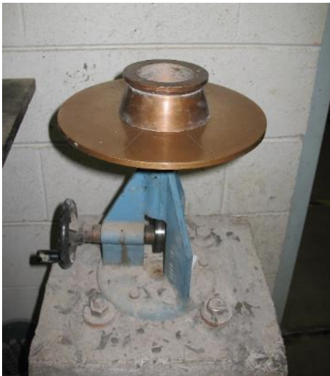
Figure 3-2: The flow test was used to determine the rheology of UHPC.
