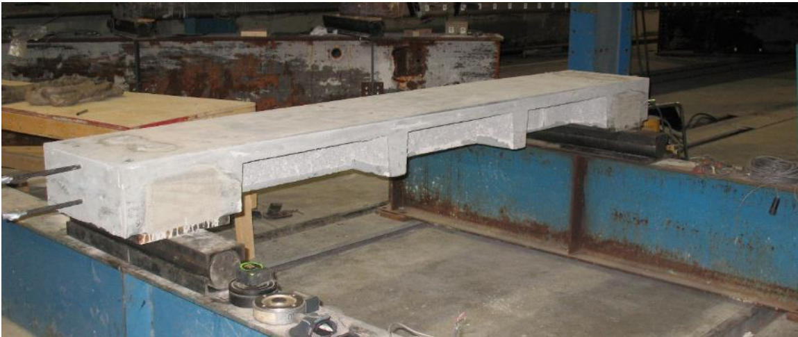
Figure 3-47: Deck sections were constructed and experimentally tested.
