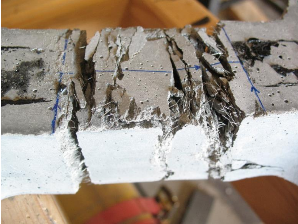
Figure 5-22: Failure surfaces revealed multiple straight cracks at failure with bridging fibers (0.4ft-2).
