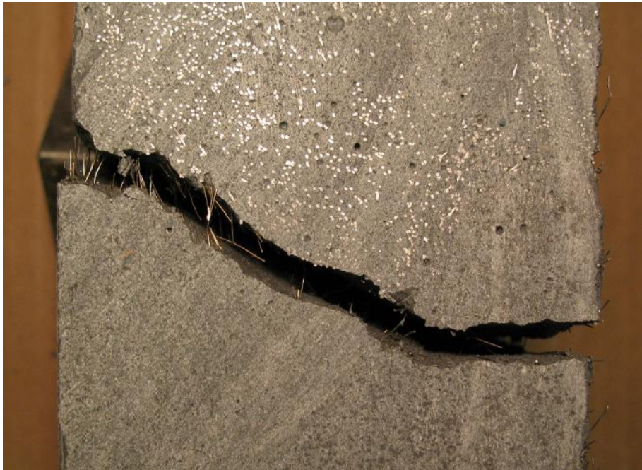
Figure 6-27: Failure crack of CP-D1 (top of web).
