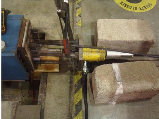
Figure 3-56: Prestressing steel was tensioned using a hydraulic cylinder while chucks and spacers anchored the tensioned steel.
