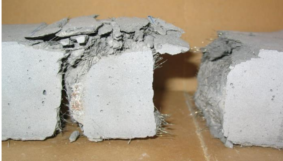
Figure 5-14: Pure compression failure of untreated UHPC with random fiber orientation (PC-2).
