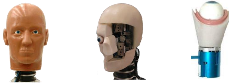
Figure 3. The FOCUS headform (left) is an advanced anthropomorphic test device that has eight facial bone segments (middle) and two eyes (right) instrumented with load cells.
