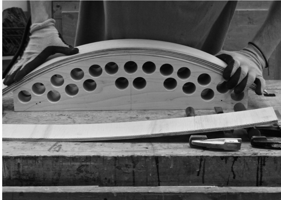
K _ Laminates bent for back, digital photo, credit / Chris Taylor
