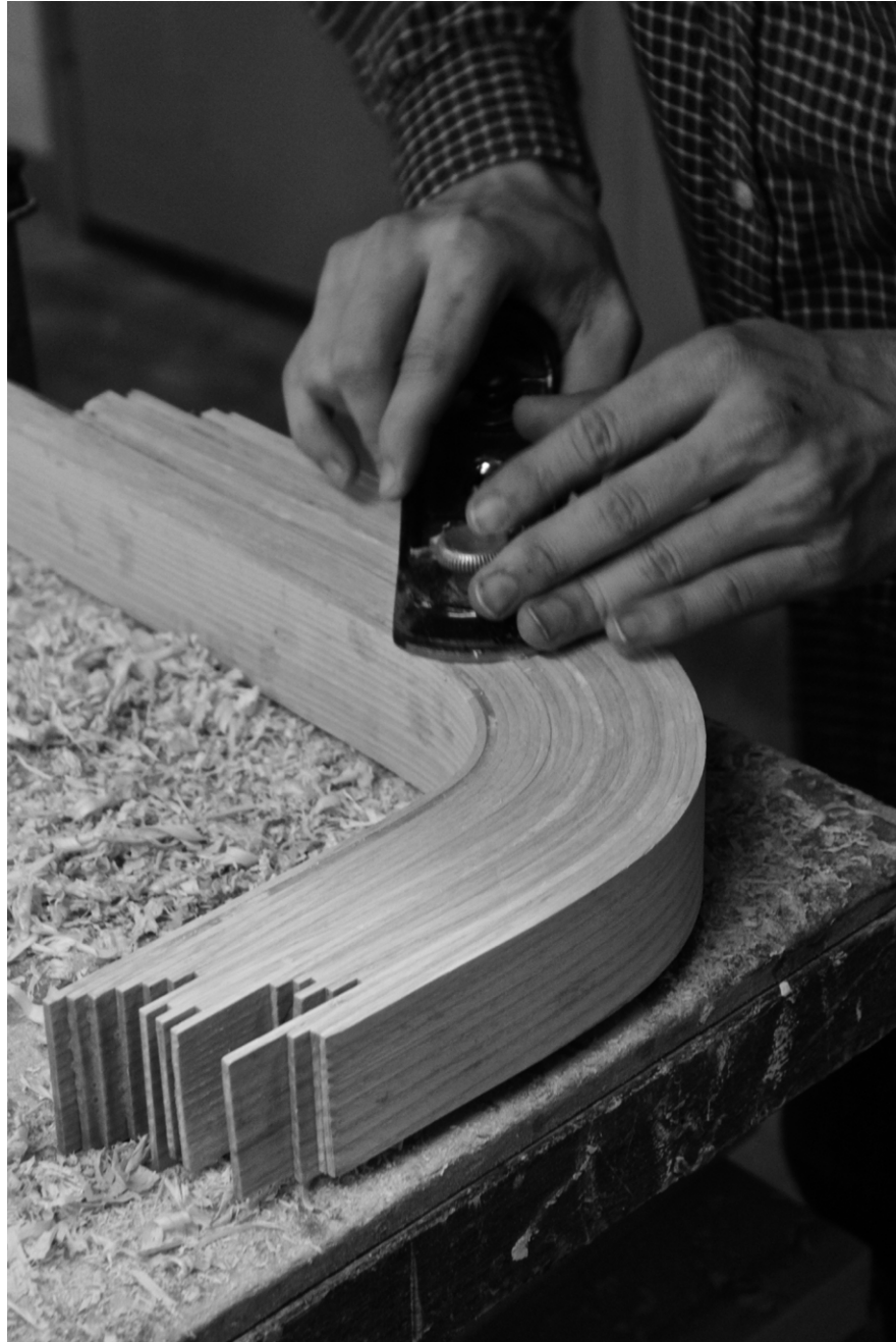
Q _ Planed surface of rear knee, digital photo, credit / John Eskeland
