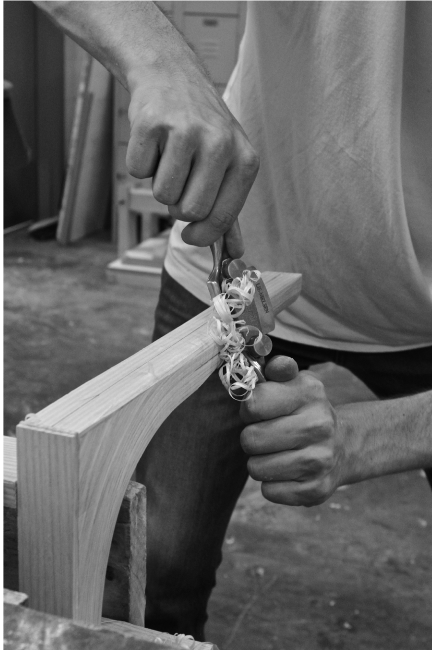
Z _ Shaping of front leg, digital photo, credit / Chris Taylor
