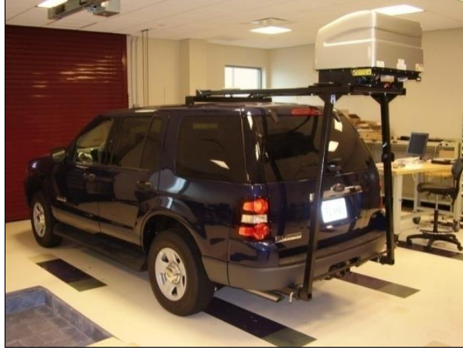
Figure 2.2. Optical terrain measurement system with inertial navigator
