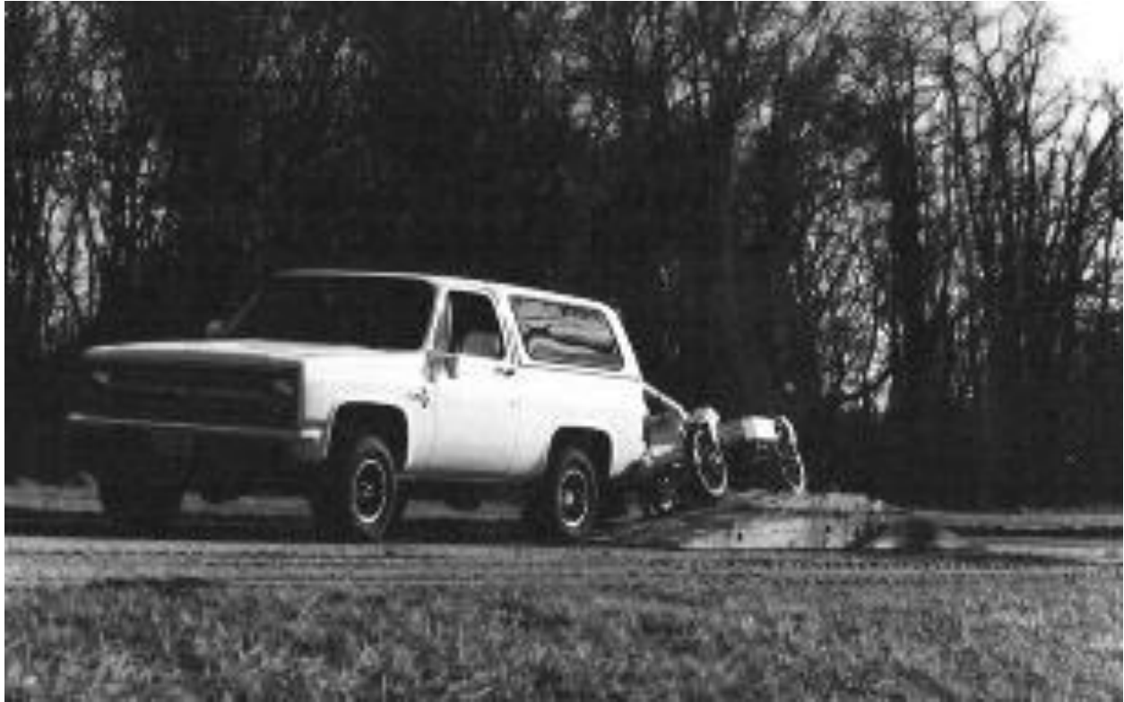
Figure 2.1. ATC profiler: example of vehicle response measurement system [15]
