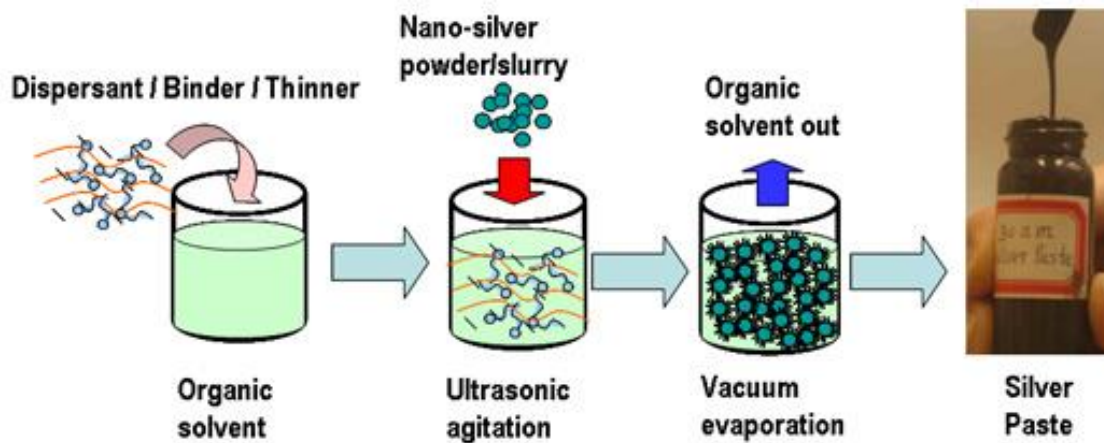
Figure 3. Preparation procedure of nanoscale silver paste. ([5] G. Q. Lu, J. N. Calata, Z. Zhang, and J. G. Bai, “A lead-free, low temperature sintering die-attach technique for high-performance and high-temperature packaging,” in Proc. 6th IEEE CPMT High Density Microsys. Design Packag. Comp. Failure Anal. (HDP’04) , pp. 42–46, 2004.) Used under fair use, 2013.
