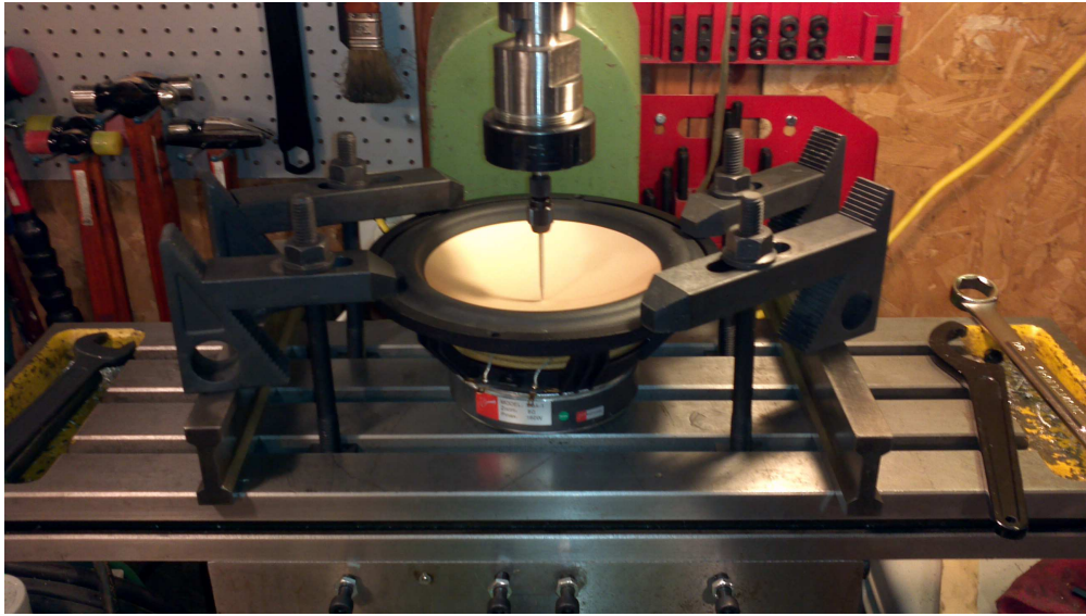
FIGURE 42. Centering the M8a Loudspeaker on the Mill
