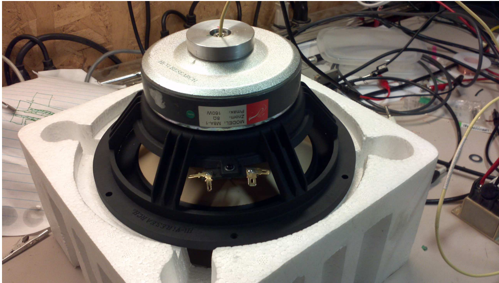
FIGURE 50. M8a Loudspeaker with Inductive Probe Installed
