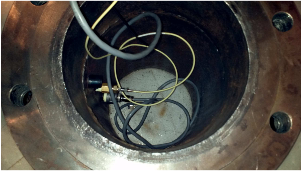
FIGURE 40. Pressure and Instrumentation Ports as Wired
