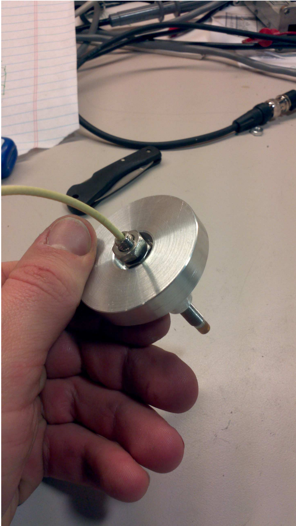
FIGURE 49. Inductive Probe and Press-Fit Fixture
