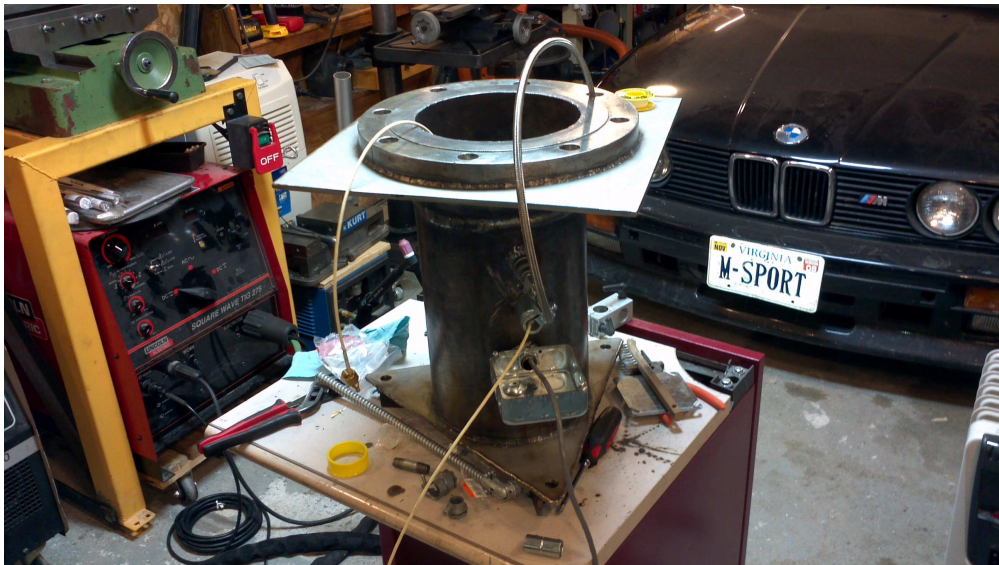
FIGURE 37. Plumbing and Wiring of Bottom Pressure Cavity
