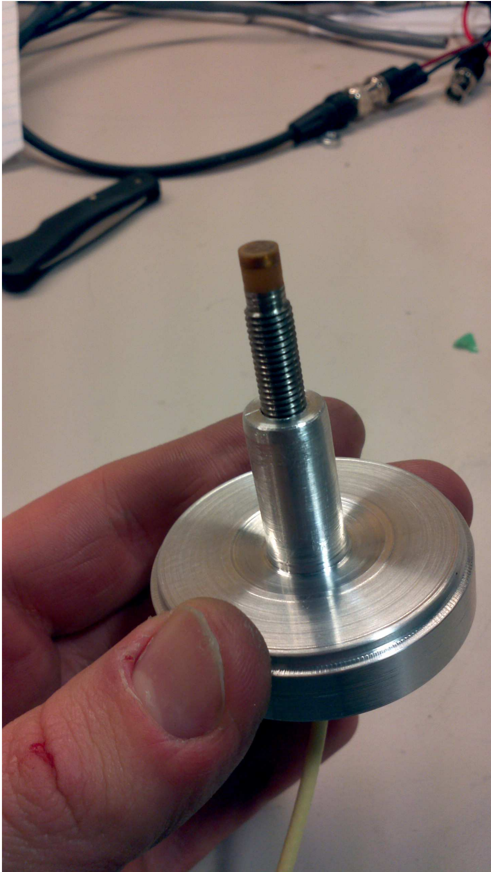
FIGURE 48. Inductive Probe and Press-Fit Fixture
