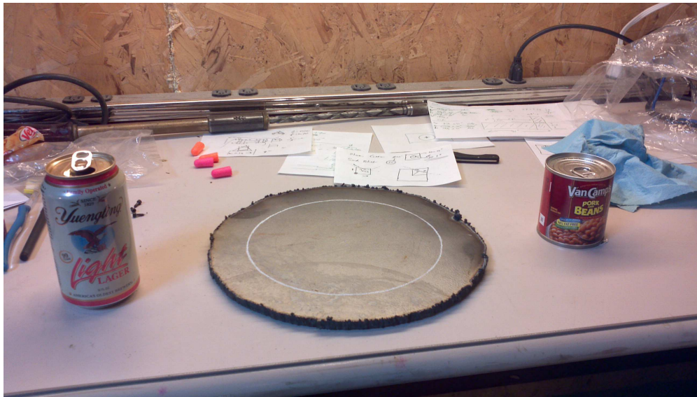
FIGURE 38. Layout and Plasma Cutting of the Paramagnetic Loudspeaker Flange
