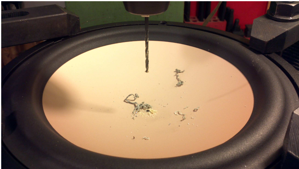
FIGURE 43. Drilling a Hole for the Inductive Probe Target
