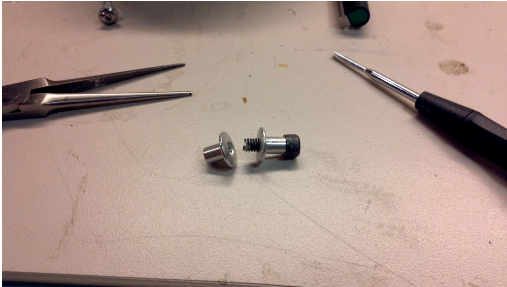
FIGURE 45. Close-Up View of the Inductive Probe Target
