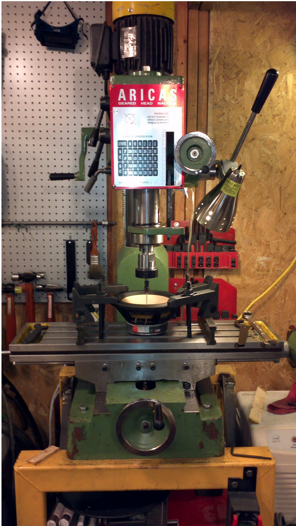
FIGURE 41. Centering the M8a Loudspeaker on the Mill
