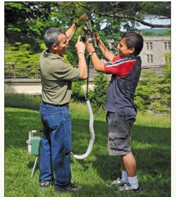
John Seiler and doctoral student Marco Yanez train with the Li-Cor 6400, a portable photosynthesis system used to measure carbon fluxes in forested ecosystems.
