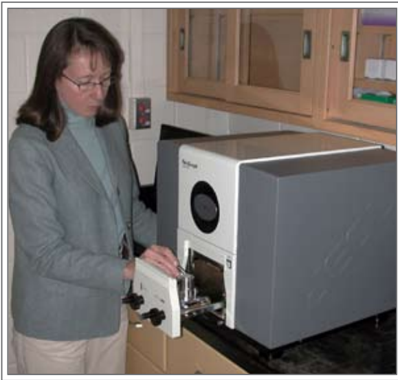
Audrey Zink-Sharp placing a specimen of balsa wood into the microscope chamber.
