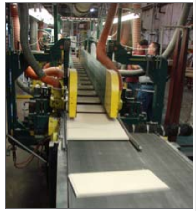
Picture 4: Gravity slide at Drawer Front DET for reduction of change-over time.
