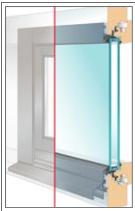
Figure 1: European wooden window with outside aluminium cladding (source: Baumgartner Fenster).
