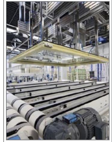
Figure 5: Automated material handling systems (source: Baumgartner Fenster).
