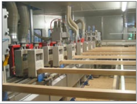
Figure 3: Automated wooden windows frame machining line (source: Baumgartner Fenster).
