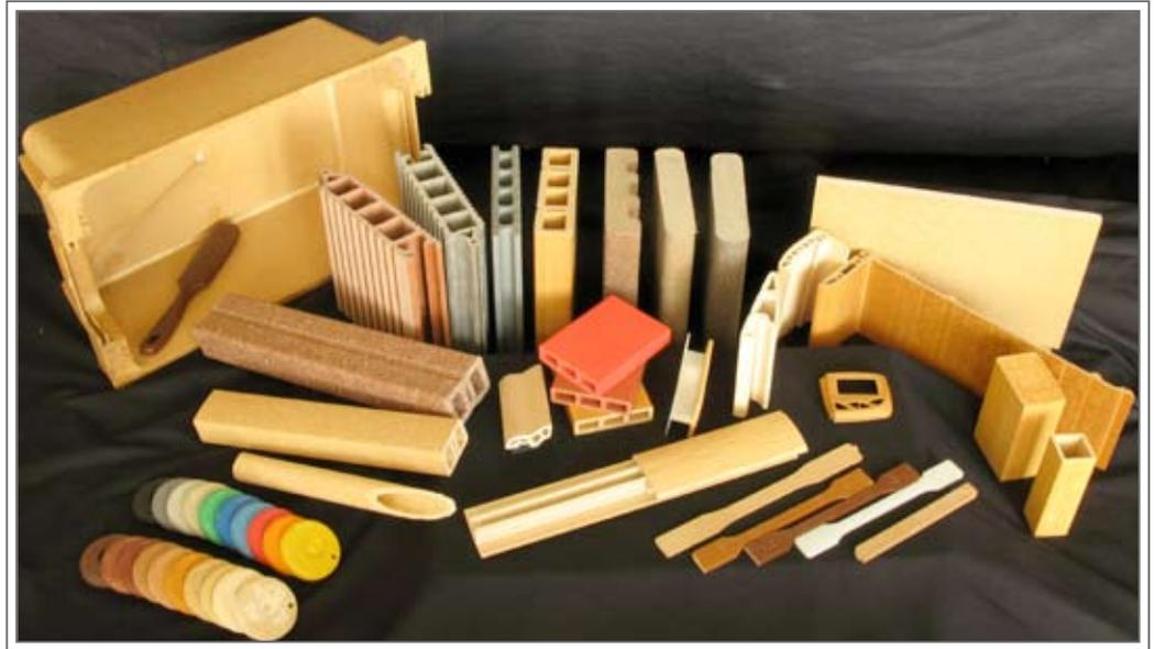
Sample products made from wood polymer composites.
