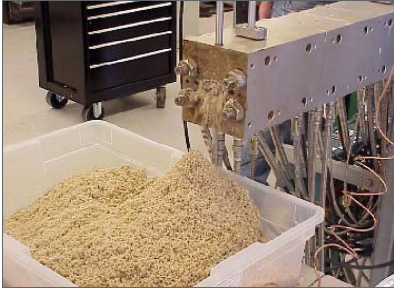
The company's grinder turns the wood pulp into a mash that can be broken down further into glucoses.
