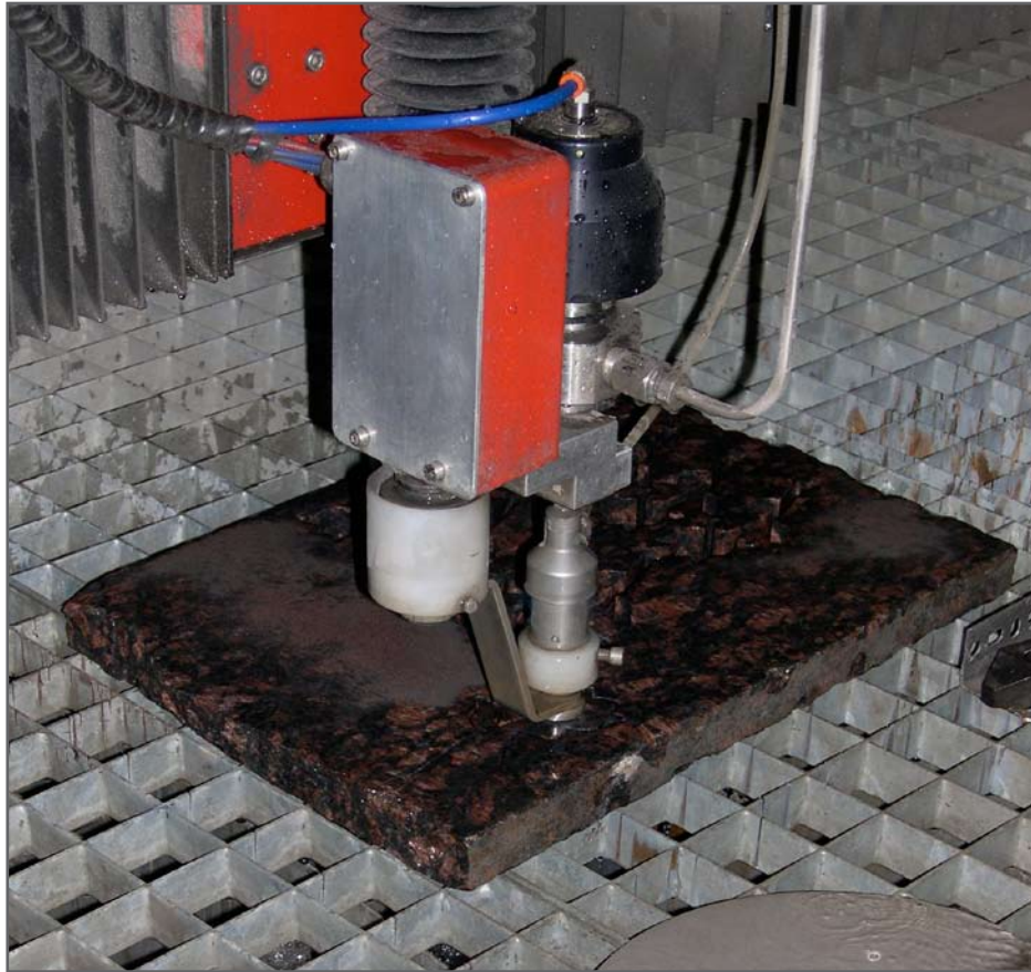
Rich Brusnahan demonstrated the Belotti High Pressure Water Jet Cutting Technology – shown here cutting a rose from a granite slab.
