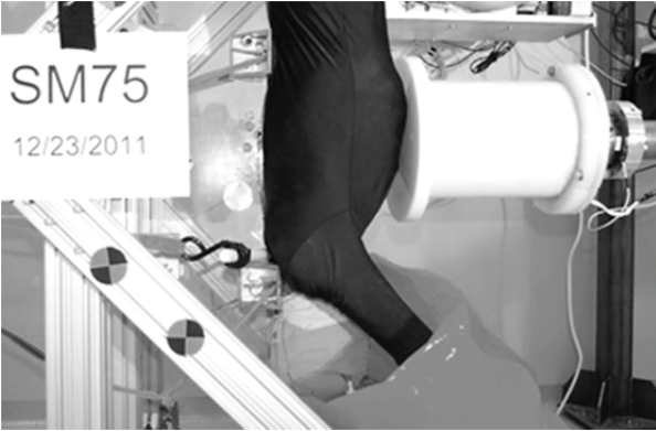
Rigid-Disk Impact at the Xiphoid Process 305-mm diameter impactor
