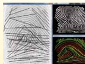
Left: Results in which a fingerprint image has been processed to detect a skeleton image (top right), then associations between ridges and minutiae have been detected (left). The same ridges have been color-coded (bottom right) to aid in visualization.
