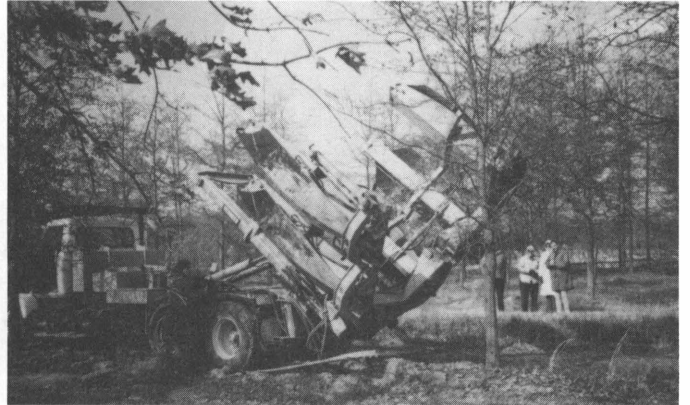
An 84" Vermeer mechanical tree digger preparing to dig a large shade tree. (Greenbrier Farms, Chesapeake, VA)
