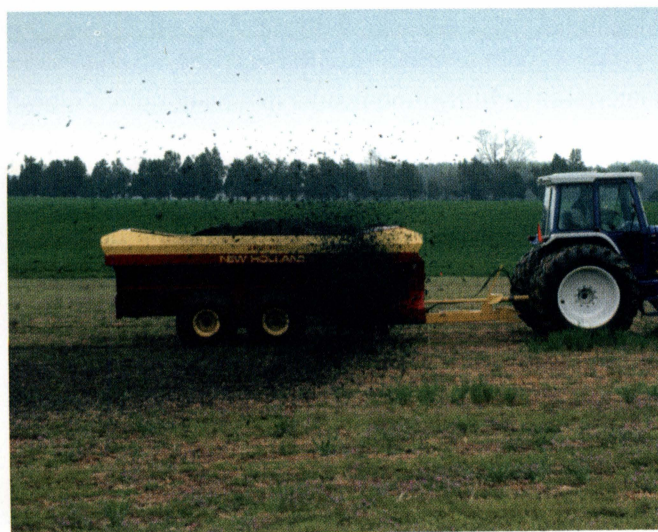
Spreading of dewatered "cake" biosolids from a manure-type spreader in preparation for planting corn
