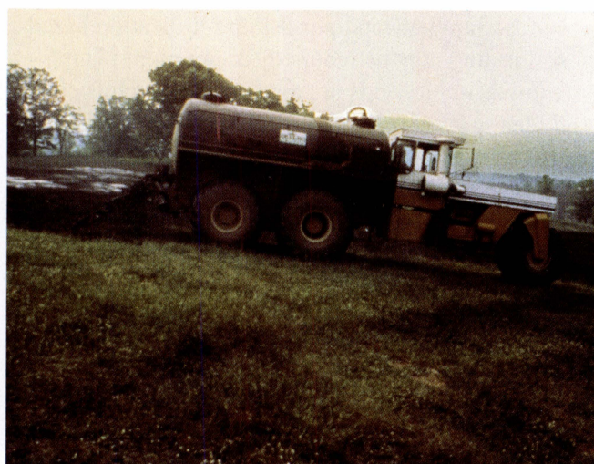
Liquid biosolids being applied to the surface of a pasture.
