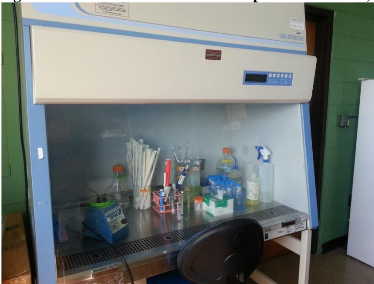
Figure A.2 Laminar Flow Hood Set-Up for Inoculation, Treatment and Enumeration
