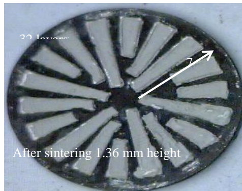
Fig. 41. Constant-flux inductor with LTCC core and DuPont Silver paste with 18 turns, 14 mm x 14 mm x 1.32 mm.
