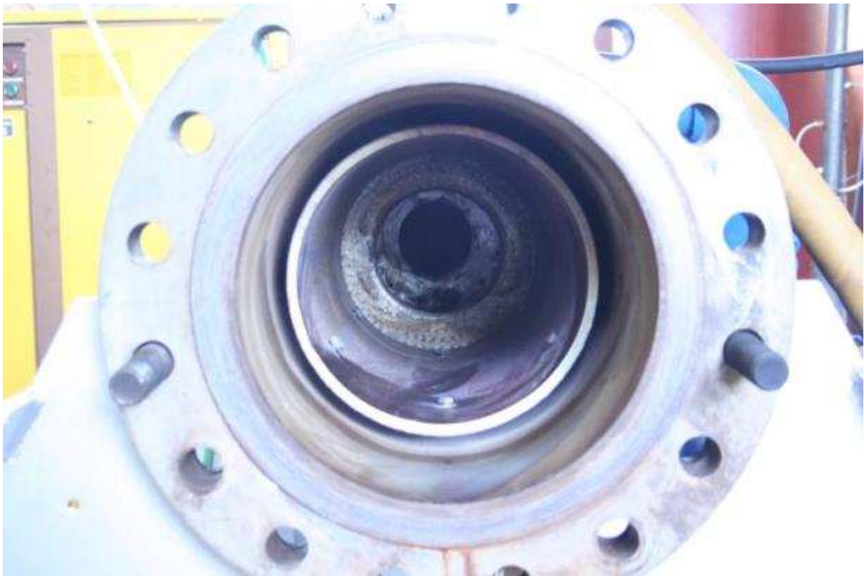
Figure 32. Picture of the stainless steel pipe insert in the burner.
