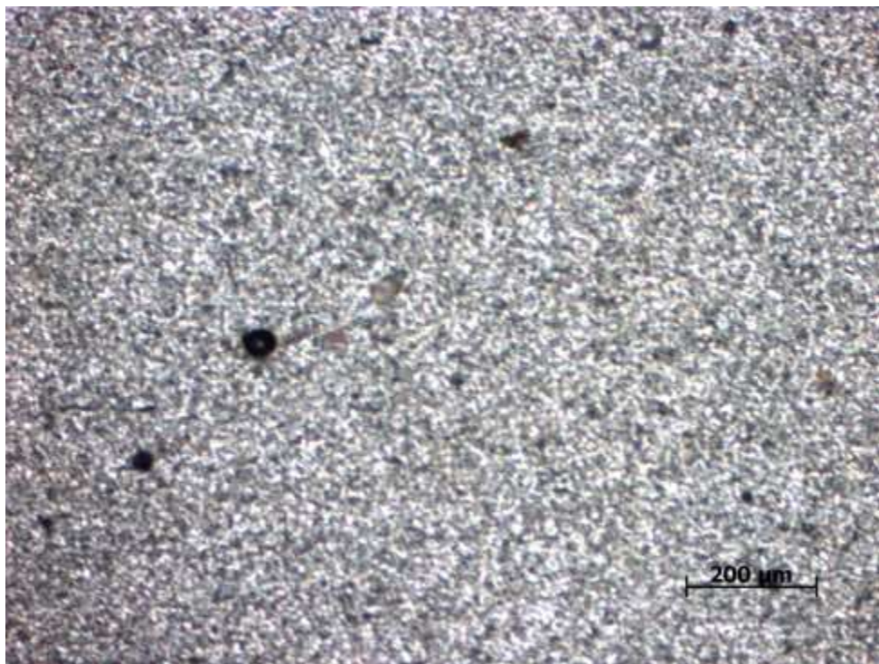
Figure 22. Sand deposition at 40° impact angle and 1273 K
