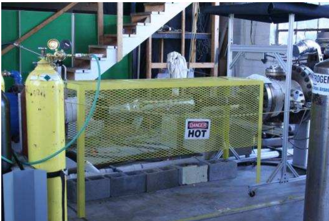
Figure 36. Picture of the safety cage
