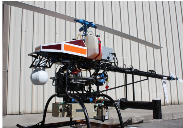
Figure 1. Sensor system components installed on an Aeroscout B1-100 helicopter.
