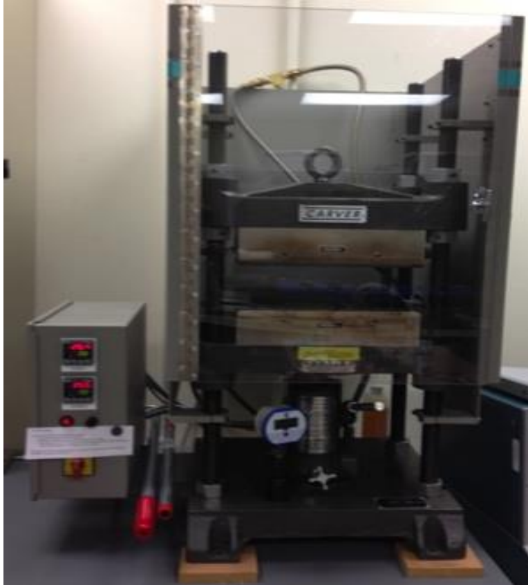
Fig. 5.2. Hot press used for applying uniaxial pressure during assembly heating.
