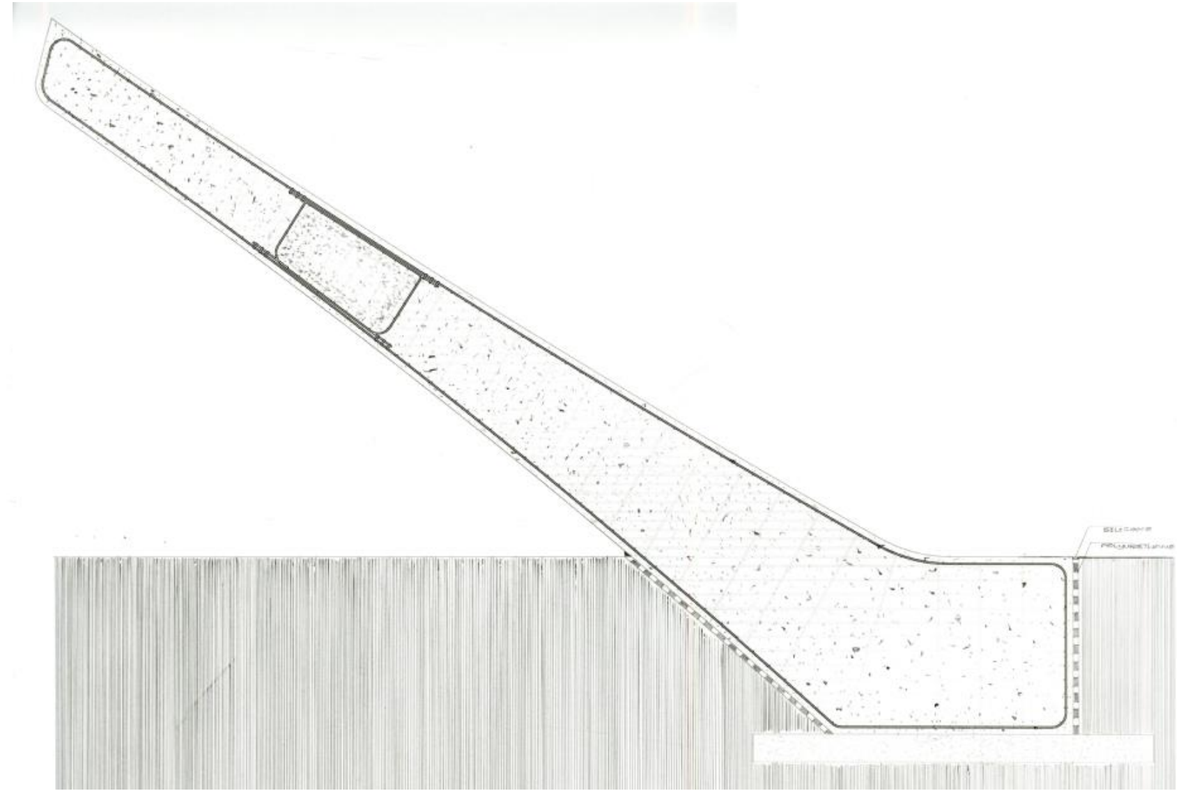
Cast-in-place foundation with pre-cast beams
