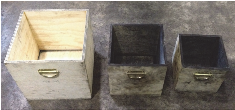
Figure 3-13. Boxes of varying size for bulk density measurement: (left) 1 \text{ ft}^3 , (middle) 0.50 \text{ ft}^3 and (right) 0.24 \text{ ft}^3
