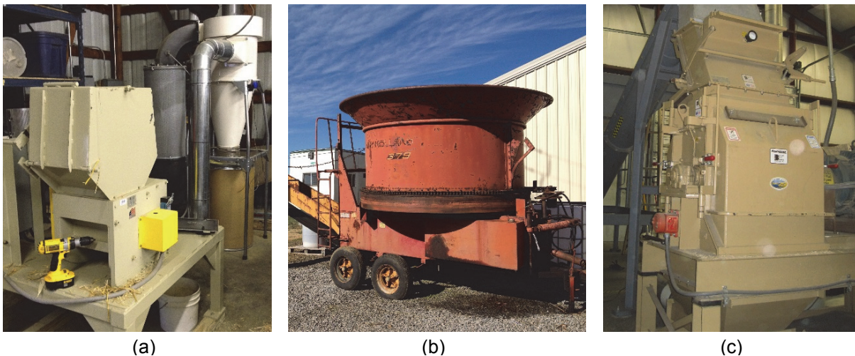
Figure 5-5. Equipment used for biomass size reduction: (a) knife mill, (b) tub grinder and (c) hammer mill
