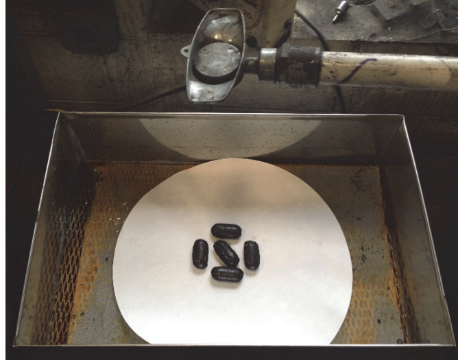
Figure 3-16. Example of briquette arrangement on filter paper for water resistance measurement
