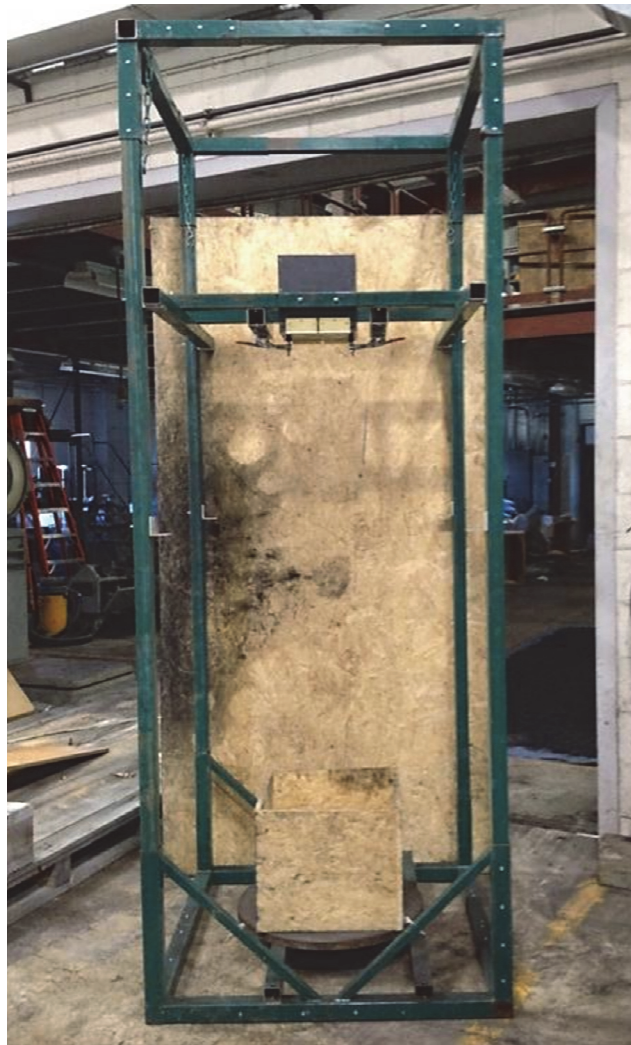
Figure 3-11. Modified ASTM shatter test device for friability testing
