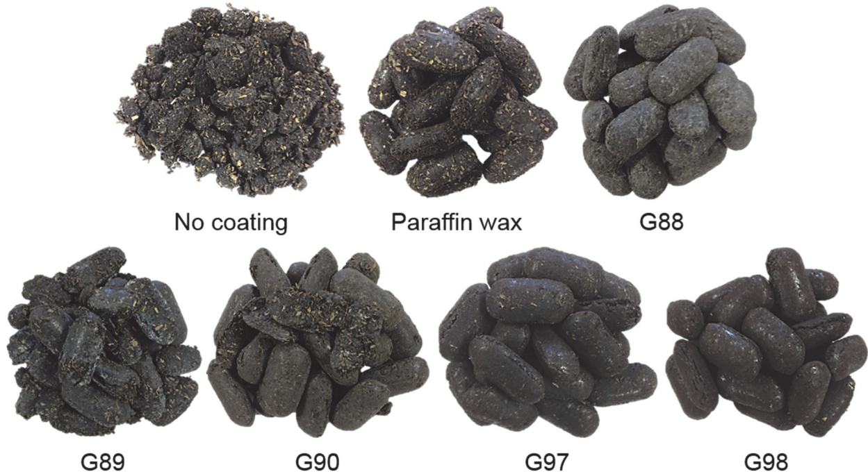
Figure 6-10. Briquette samples after durability and water uptake tests
