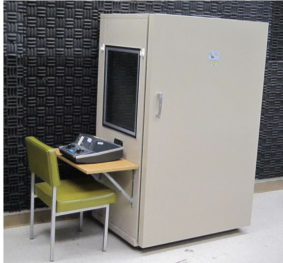
Figure 36. Industrial Acoustics Company (IAC) mini booth and Beltone 119 audiometer used for participant audiometric screening.
