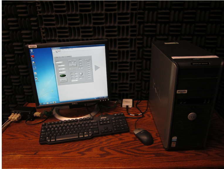
Figure 35. Experimenter control station showing from left to right, multiplexer (black project box), experimenter screen, DAQ (white box), and desktop CPU.
