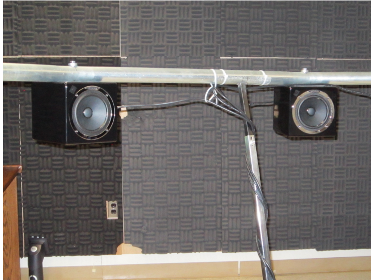
Figure 32. Behrtone C50A speakers, suspended from custom fabricated metal structure, facing the listener position in the center of the circle (acoustically-transparent fabric, used to conceal speakers, removed here for photo).
