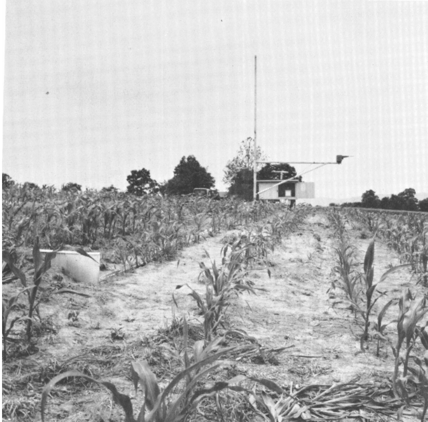
Figure 3 - Surface runoff measurement plot with net radiometer installation in the background.
