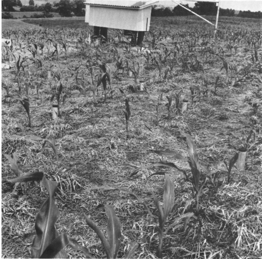
Figure 5 - Excess tube design for determining spatial variation of soil moisture.
