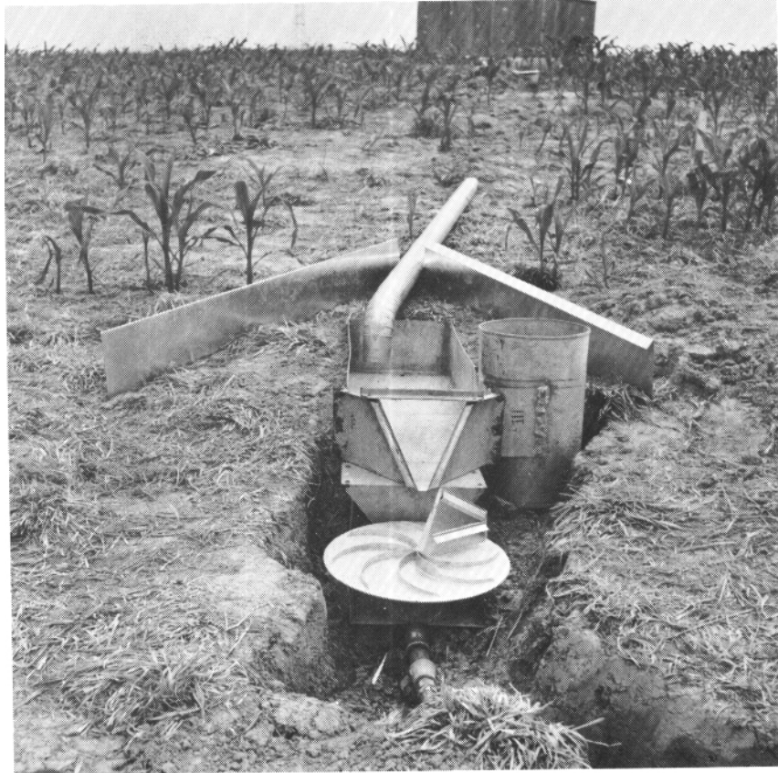
Figure 4 - H-type flume with soil sampler attached.
