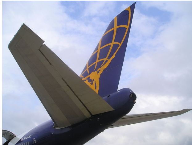
Figure 6.2: Photograph of an empennage, or tail assembly, from a typical modern transport aircraft
