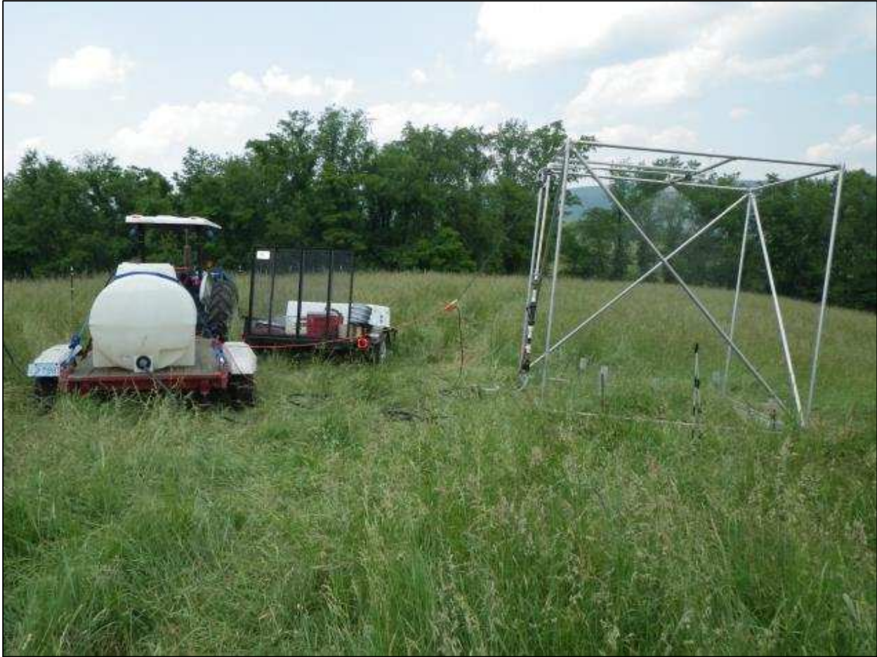
Figure 3.16. Rainfall simulation. Tank of source water (left), simulator (right).
