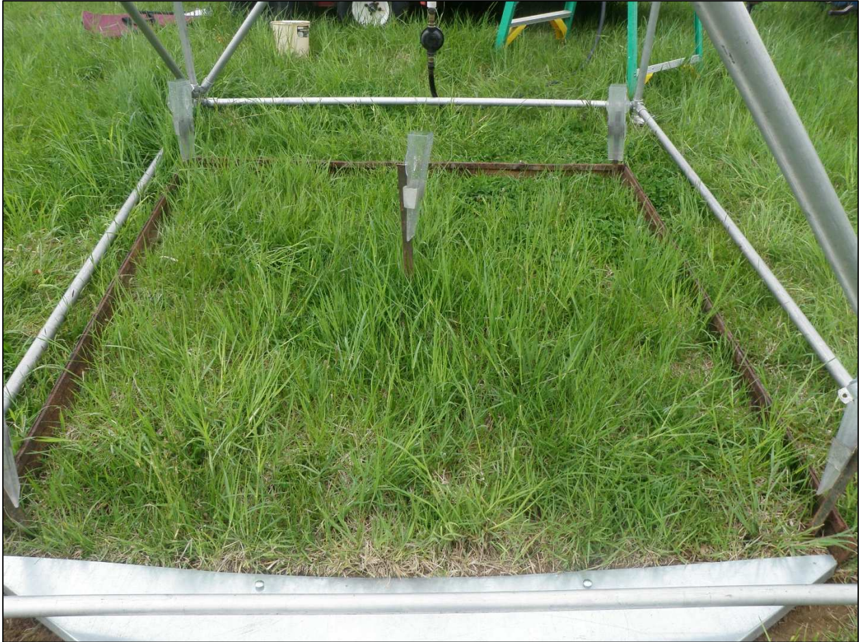
Figure 3.15. Runoff plot borders, collection flume, and rain gauges within frame of rainfall simulator.
