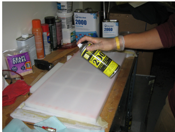
Figure A3: Applying the Mann Ease Release 200 to the HDPE mold.
