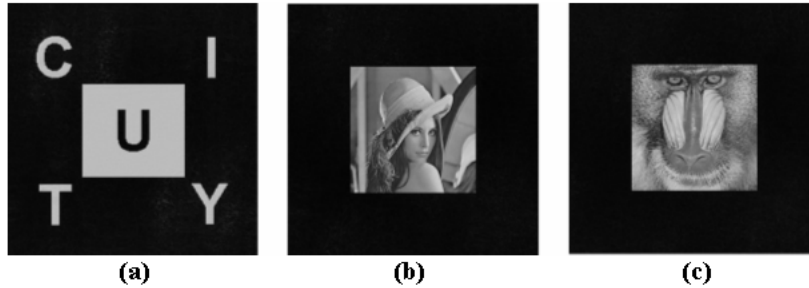
Fig. 4. (a)-(c) Reconstructed images of the phase-only holograms derived from our proposed unidirectional error diffusion method.
