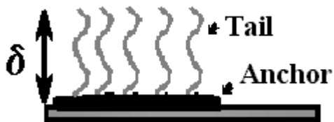
Figure 2.16: Schematic of block copolymer adsorption with and adsorbed anchor and an extended tail with a thickness \delta .
