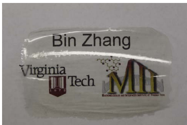
Figure 4.20 Picture of a typical trans -1,4-cyclohexylene containing PAES film sample by solvent casting
