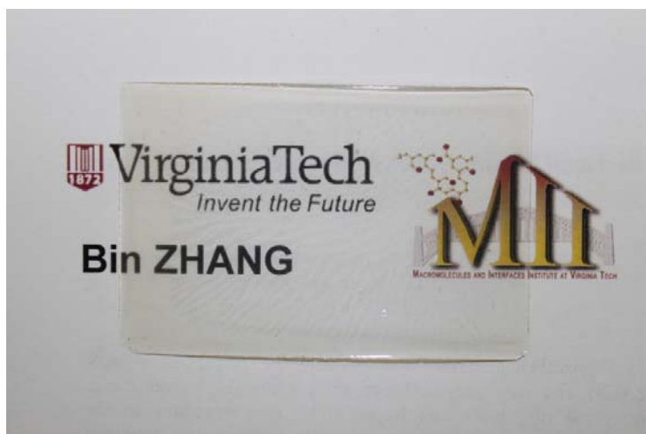
Figure 5.3 Picture of a typical trans -1,4-cyclohexylene containing PAES film sample by solvent casting
