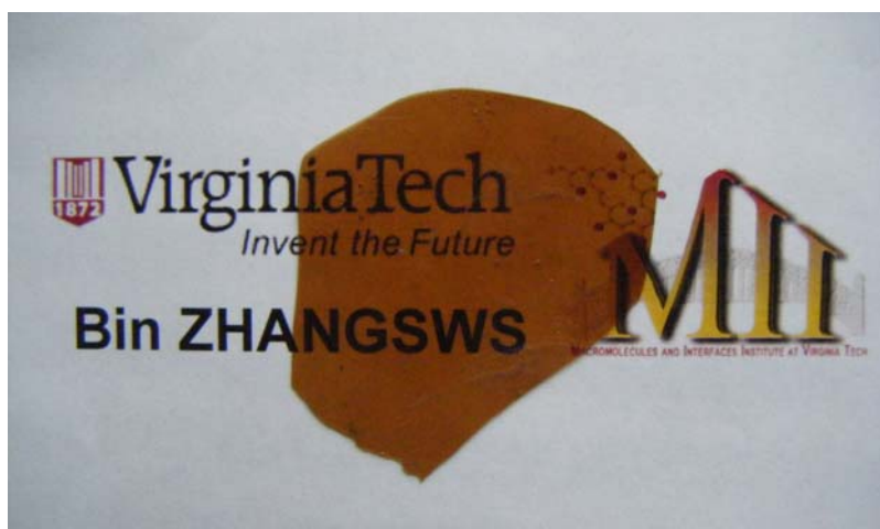
Figure 4.19 A typical film sample by compression molding
