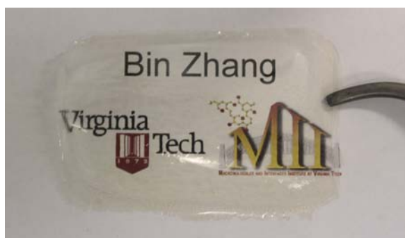
Figure 3.11 Picture of a typical CMB based PAES film sample by solvent casting
