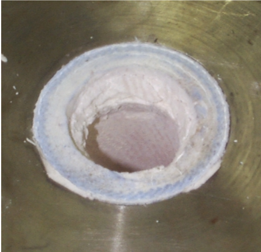
Figure 4.18: Failure mode of flange in a compression test: circular cracks
