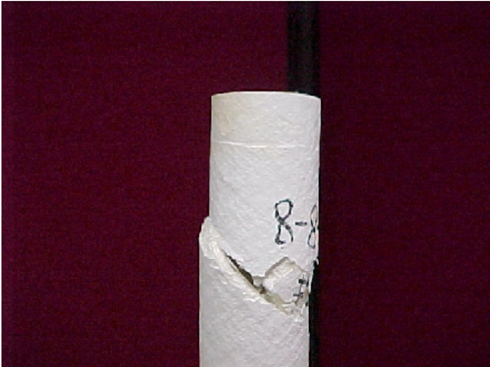
Figure 2.27: Failed four-point bend test specimen.
