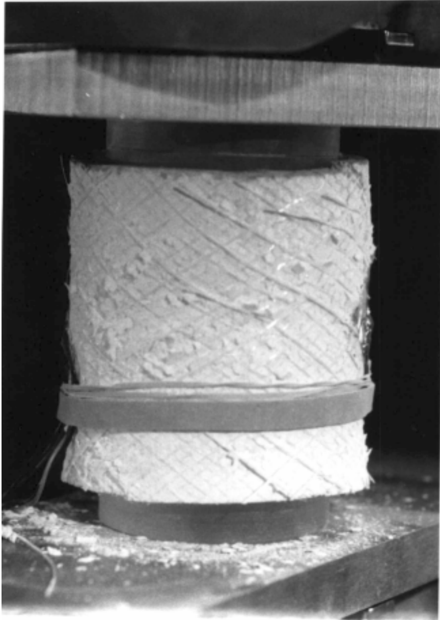
Figure 2.11: Failure sequence in a burst test: No. 4
