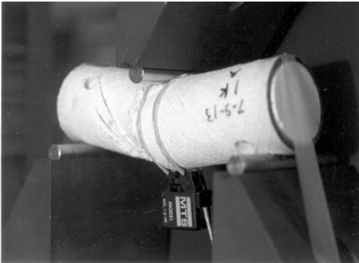
Figure 2.22: Three-point bend failure sequence: No. 2 (side view)
