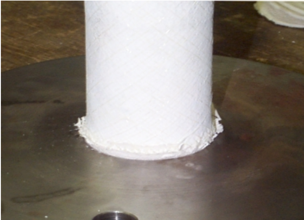
Figure 4.19: Failure mode of flange in a compression test: torn surface layer
