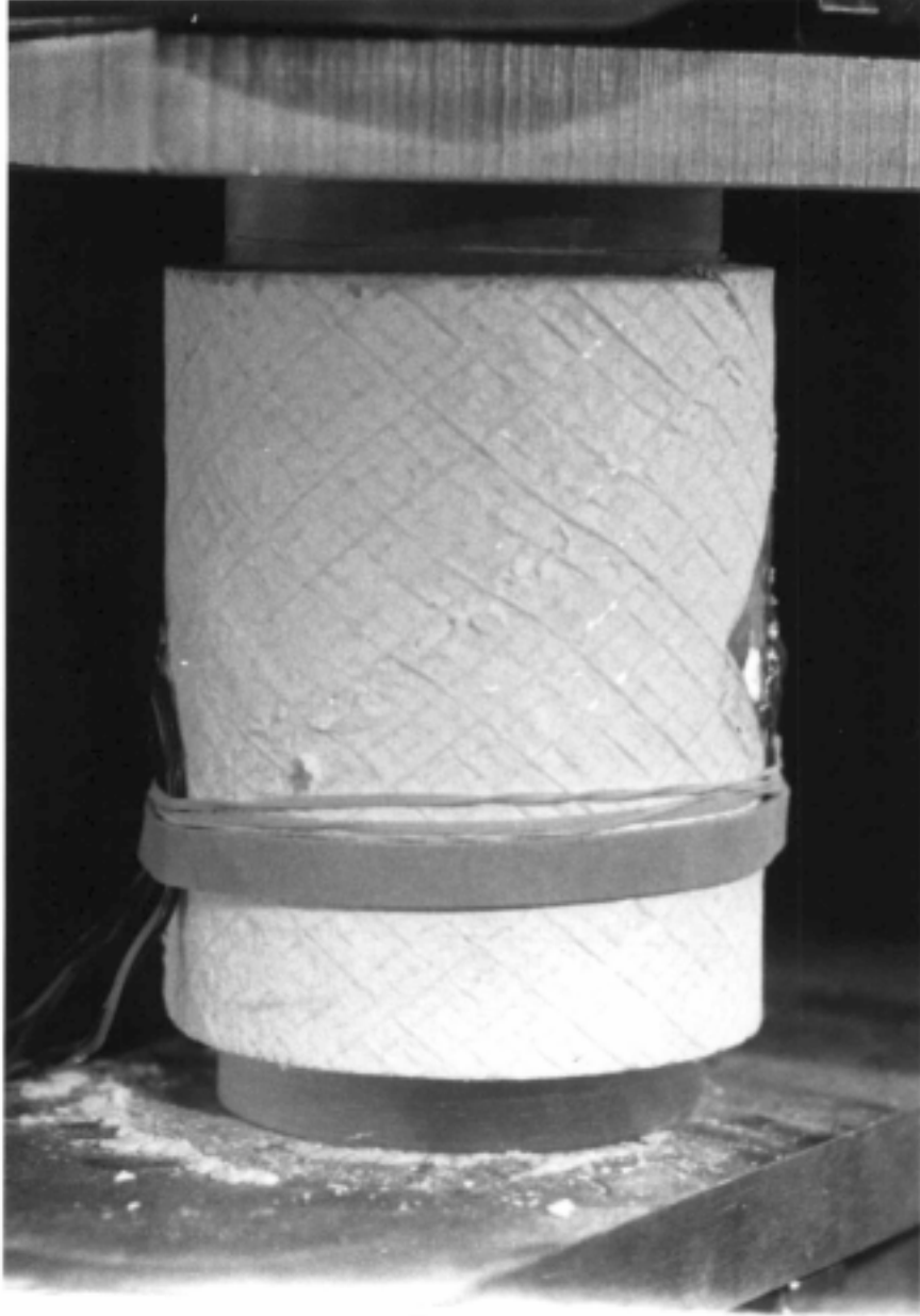
Figure 2.9: Failure sequence in a burst test: No. 2
