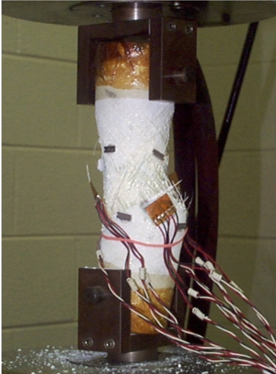
Figure 2.15: Tube tensile failure mode: necking and stretching
