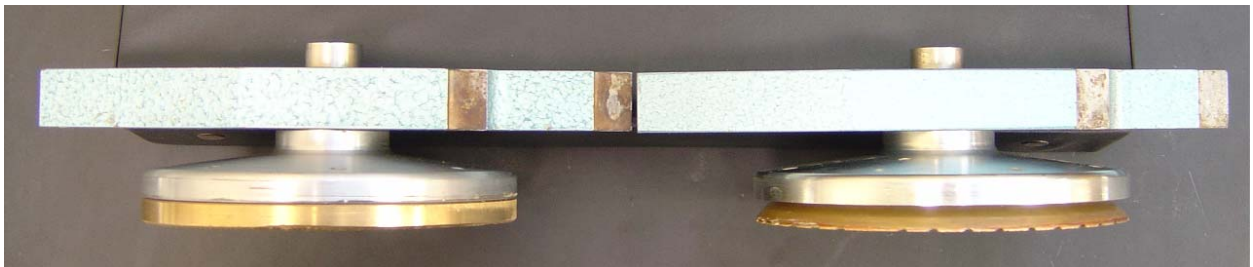
Figure 4-6. Side view that shows the difference between the original porous bronze platen (on the left) and the modified porous bronze platen (on the right).
