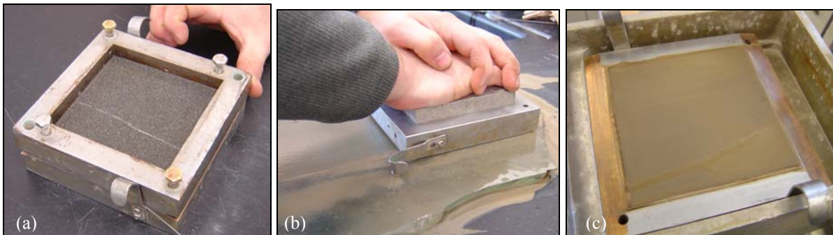
Figure 5-4. Preparing a direct shear test specimen; (a) wire-cutting a direct shear specimen, (b) rubbing the cut plane on frosted glass to align clay particles, (c) the polished failure plane.
