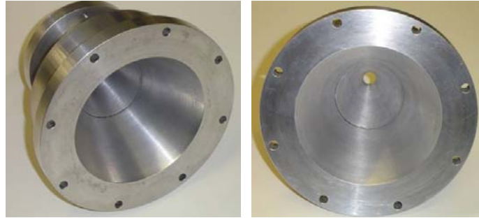
Figure 4-5. Reducer - used to reduce diameter from 101.6 mm to 10 mm
