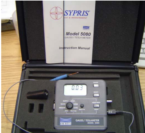
Figure 4-8. Gauss-meter and "ultra-thin" transverse probe
