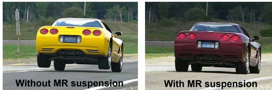
Figure 2-5. Base C5 Corvette and 50th anniversary Corvette with Magnetic Selective Ride Control suspension (image adapted from [17])
