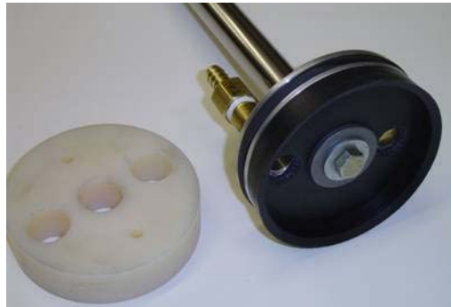
Figure 4-4. Piston with Viton ® o-ring and nylon bushing
