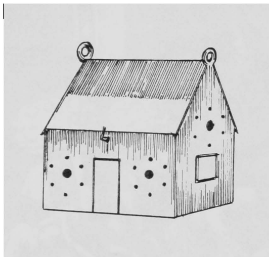
Figure 17. A safe described by Randle Holme as " a kind of little house made of wood and covered with haire cloth, and so by two rings hung in the midle of a Rome, thereby to secure all things put therein from the cruelty of devouring Rats, mice, Weesels, and such kind of Vermine. Some have the pannells of the Arke made all of Tyn, with small holes for aire; others of woode" (p. 17). Drawn from illustration 88 facing p. 18.
