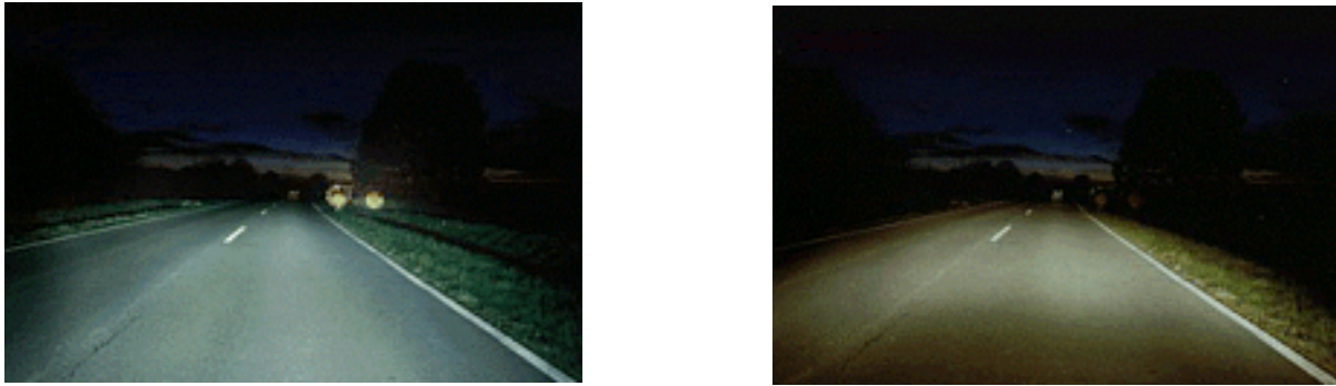
(a) (b) Fig. 1.1. Comparison of road conditions with different headlamps [B2]: (a) 35W HID lamp and (b) 55W conventional lamp.
