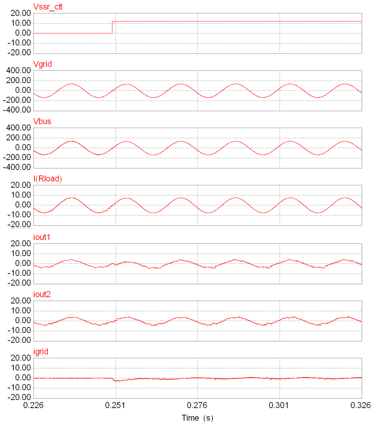
Fig. 3.9. Islanding mode to grid-tie mode transfer simulation results.
